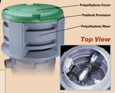
Liberty's installation kits provide all the components for a professional installation inside the riser. Kit includes: JB-Series wiring box and hardware, check valve with a disconnect union feature, coupling and elbows (PVC piping not included). Kits available in 2" discharge and vent size only.
