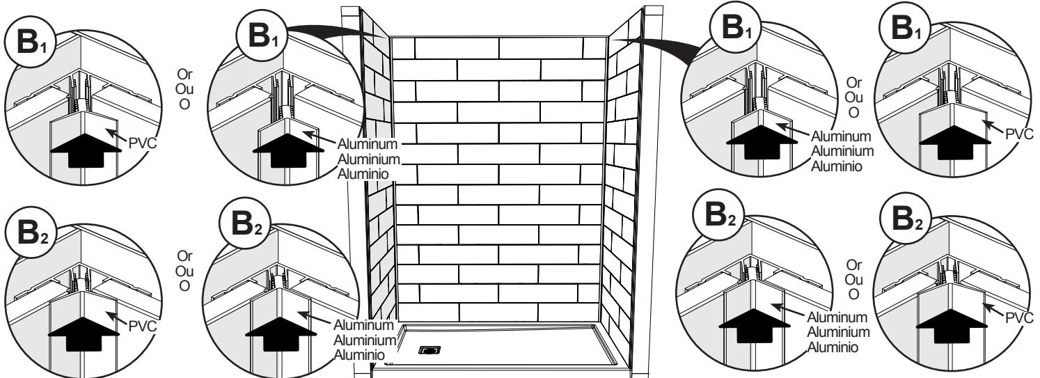
C. Apply beads of silicone on both exterior edges of the each wall, where the edge trim will fall.
