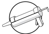
**A.** Apply beads of silicone on each side of both wall trims as shown.
