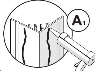
A. Apply a bead of silicone behind the corner trim. Place the trims at the corners of the alcove. Drill holes and countersink with a countersink bit. Fasten with dry wall screws.
