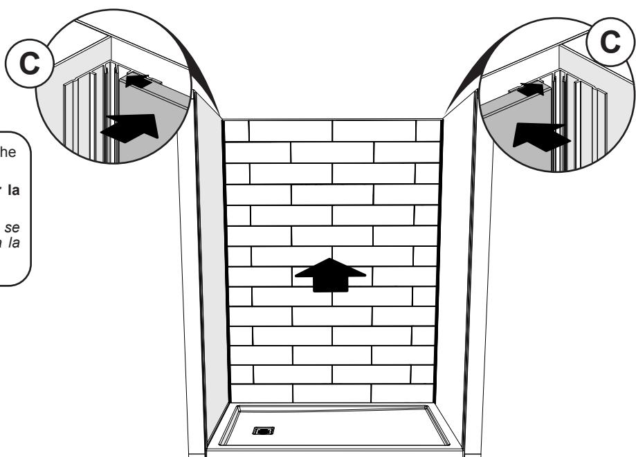
D. Repeat for the side walls. Press firmly the panels against the wall.
