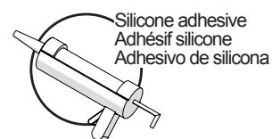
A. Apply beads of silicone on both edges of the either the aluminum or PVC middle trim piece,
