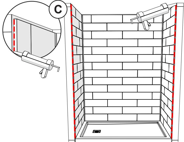
D. Insert the edge trim piece on each side (optional). See the two ways it can be installed in the images. Apply silicone to the other missing joints as indicated in the wall installation guide.
