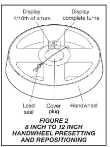
**Step 4.** Gently pull the handwheel up and remove it from the valve spindle.
