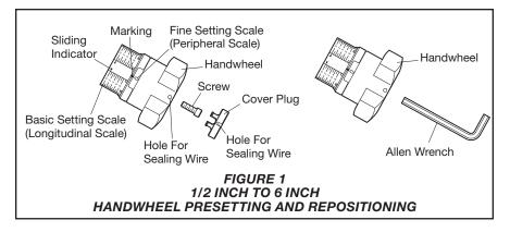
One complete turn of the handwheel adjusts the indicator one full position.
