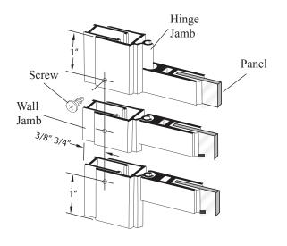
**7**When installing the 2nd panel slide the hinge jamb of the door panel assembly (H) over the mounted wall jamb (B) so the door will open outward while holding the panel, install the snap-n-fill (J) into the header. This will allow you to adjust the 2nd door.
