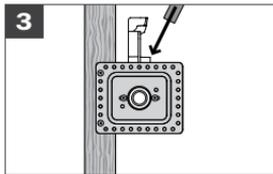
Working from the back, push 1/2" PEX through LockBlock and plate then carefully secure tube in bend support making sure not to kink the tube.
