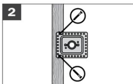
Secure Face Plate to structure with two screws.
