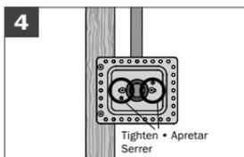
Complete the installation by tightening all screws to prevent movement.
