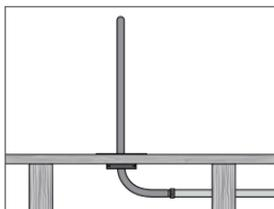
For floor penetrations, secure plate to sub-floor from basement or crawlspace after drilling 5/8" hole for PEX to pass through.
