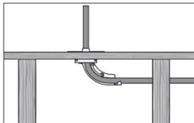
For floor penetrations, secure plate to sub-floor from basement or crawlspace after drilling 5/8" hole for PEX to pass through.
