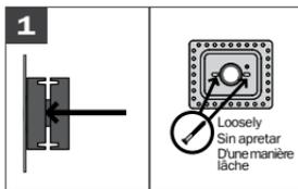
Attach pre-assembled LockBlock loosely to plate with two screws.
