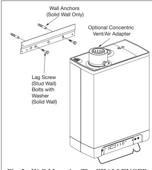
Fig. 2: Wall Mounting The CHALLENGER
