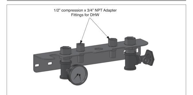
Fig. 10: Installation of Domestic Compression Adapter Assemblies
