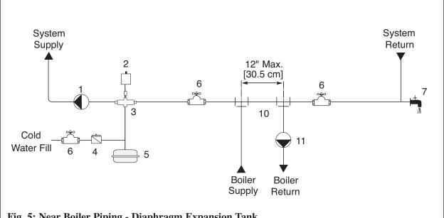
Fig. 5: Near Boiler Piping - Diaphragm Expansion Tank
