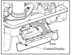
Fig. 17: Accessing Low Voltage X4 Connections
