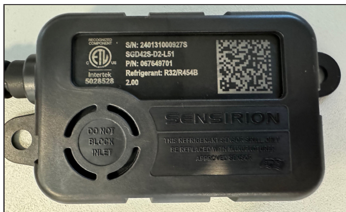
FIGURE 22. Example of Clear, Unobstructed Sensor Inlet
