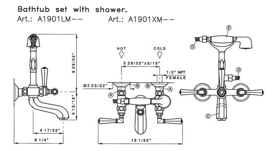
Notes: Faucet must be installed a minimum of 2 inches above fixture rim. Install per local codes. Faucet must be installed with a listed in-line anti-scald device.
