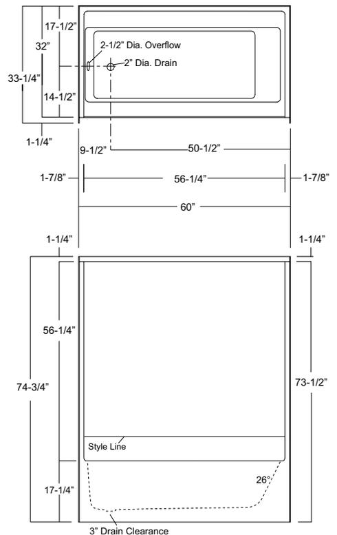
**Illustration 1b - End Drain, Unit Dimension & Alcove Framing Guidelines (dimensional tolerance + / -1/8")**
