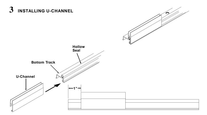
Trim excess hollow seal off each end of bottom track.
