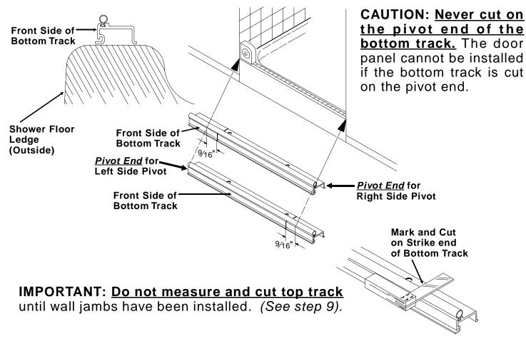
To determine the pivot end, position the bottom track near the ledge with the front side of track toward the outside of shower.
