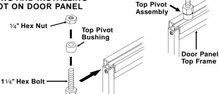
Insert the top pivot bushing over the 11/4" bolt and partially thread the 1/4" hex nut on the bolt.
