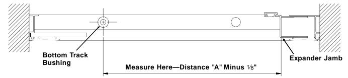
Position the door panel so that the strike side with magnetic strip is toward the expander jamb.
