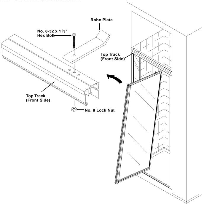
Lift the door panel and insert projecting bolt into bushing in bottom track. Slide the pivot block in top track and tilt door panel so that the projecting bolt at top engages in <u>larger</u> hole in pivot block.
