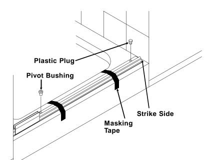
Insert the plastic plug into the hole on the strike side of the bottom track. Insert the pivot bushing into the hole on the pivot side of the bottom track.
