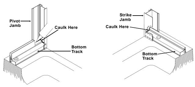
Apply a bead of caulk where the pivot jamb and strike jamb meets the bottom track.
