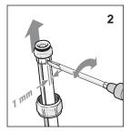
Use a screwdriver to open clamp ring and remove fitting
