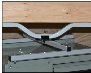
Photo #1 (On left) Close-up of Circular Adjustment Plate with locking hardware.
