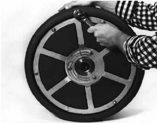
Figure 23 – Removing Pigtail Anchoring Bolt
