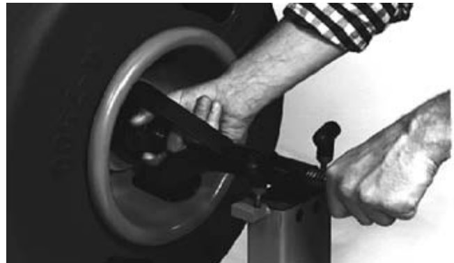
Figure 21 – Removing Knob From Center Shaft
