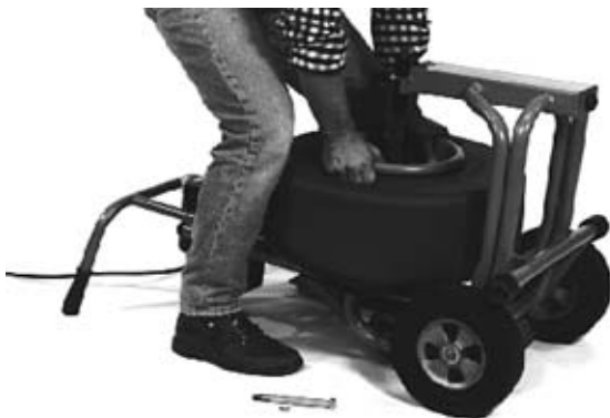
Figure 20 – Lifting Drum Assembly Onto Frame
