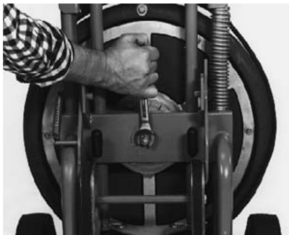
Figure 7 – Check Bolt to Ensure Tightness
