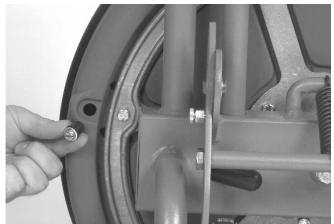
Figure 13 – Drum Drain Hole
