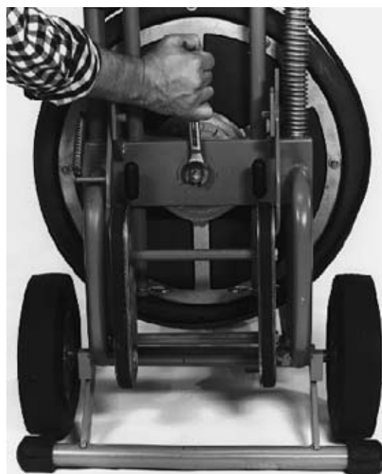
Figure 19 – Removing Rear Support Bolt
