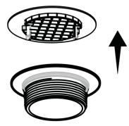
3. Cut the outlet tube into the suitable height, to match the shower base.
