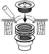
4. Glue the outer edge of the outlet tube, then fix the floor drain to the tube.
