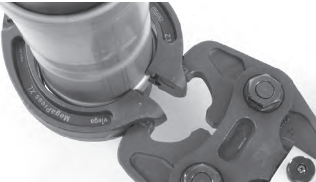
Figure 12 – Attaching Actuator to Press Ring
