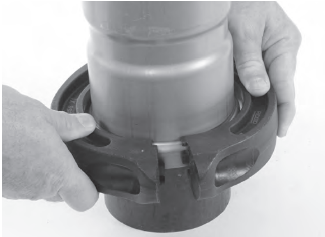
Figure 11 – Installing Press Ring Onto Fitting
