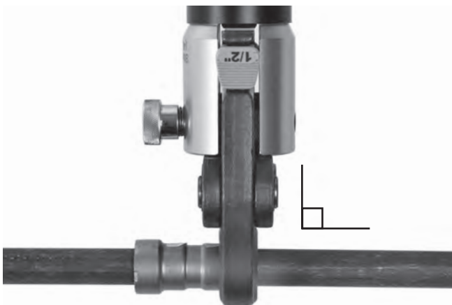
Figure 10 – Jaws Appropriately Placed
