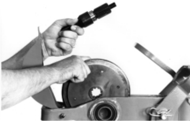
Figure 12 – Remove Cutter Wheel Assembly
