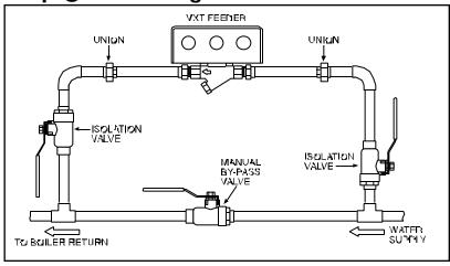
Feeder must be installed with a manual by-pass. Use isolation valves and unions to allow easy removal for service or replacement.
