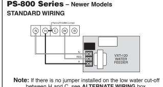
between H and C, see ALTERNATE WIRING box.
