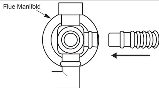
3. Fit the pipe stopper over the connection between the flue elbow and the manifold. Engage the hook and rotate it until it snaps against the body of the clamp.
