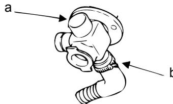
2. Connect the flue elbow to the manifold while moving the appliance into position.
