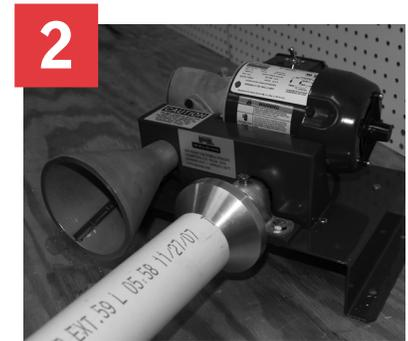
Chamfer (bevel) the end of the pipe 10° - 15°.
