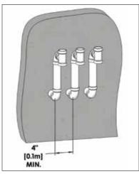
Figure 10: Sidewall vent termination - indoor combustion air applications
