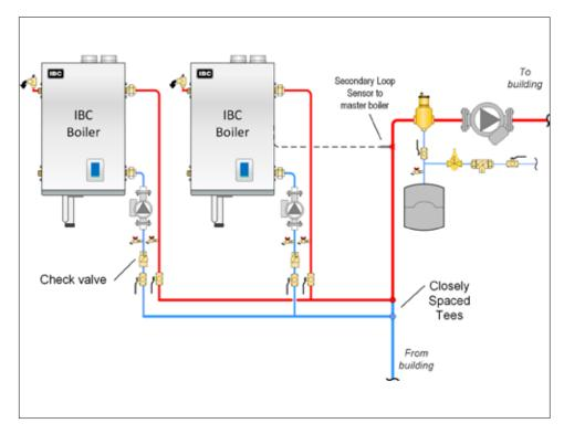
Figure 41: Multiple boiler piping concept
