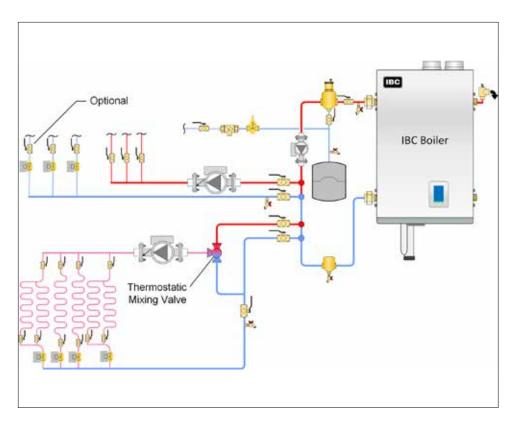
Figure 35: Typical two-temperature space heating piping concept
