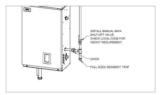
Figure 43: Typical gas piping connection
