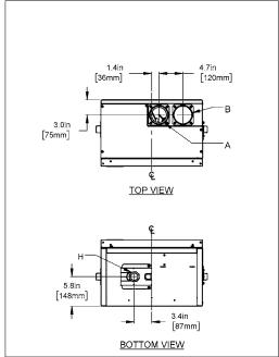
Figure 1: Dimensions / Connections for SL 14-115 G3 - Front view, side view, top view and bottom view
