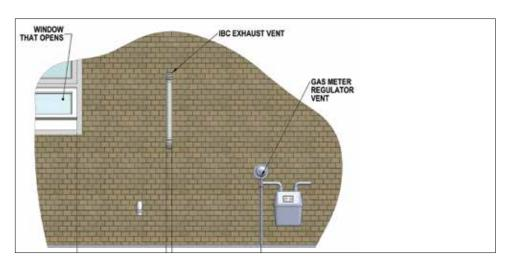
Figure 12 Vent terminal clearances
