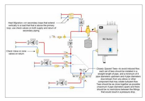
Figure 32: Important primary-secondary piping details with closely-spaced tees
