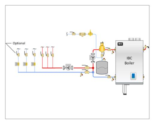
Figure 34: Typical one-temperature space heating piping concept
