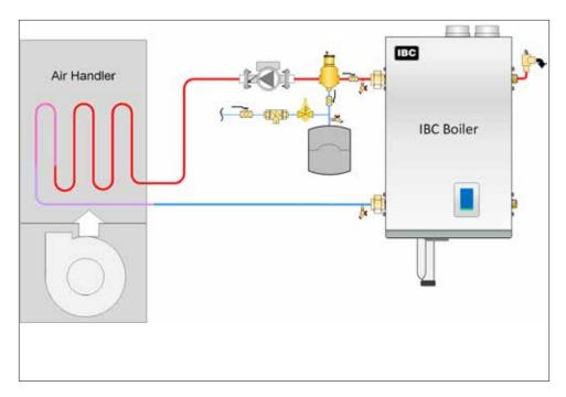
Figure 39: One pump parallel piping concept
