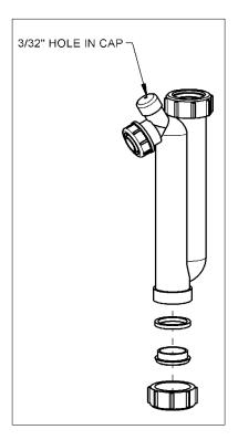
Figure 25: Condensate trap disassembly for cleaning
