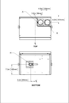
Figure 3: Dimensions / Connections for SL 30-199 G3 - Front view, side view, top view and bottom view
