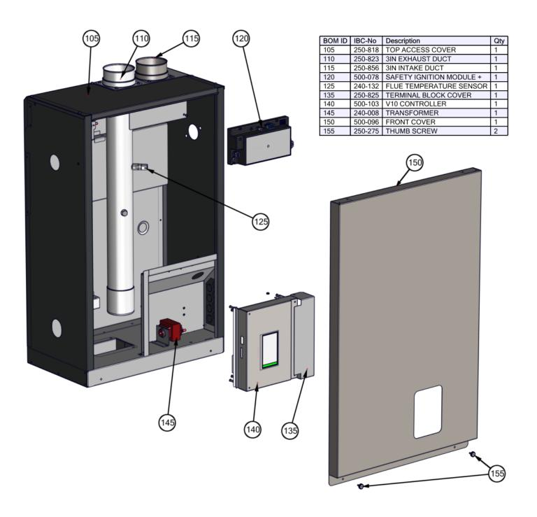
Diagram 6.1-1: Boiler assembly parts
