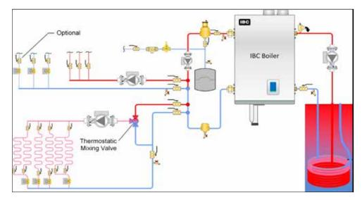
Figure 37: Two sided piping, DHW and space heating piping concept
