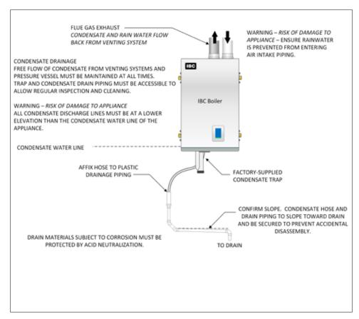
Figure 26: Condensate trap drainage
