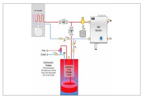
Figure 40: Two pump, two load parallel piping concept
