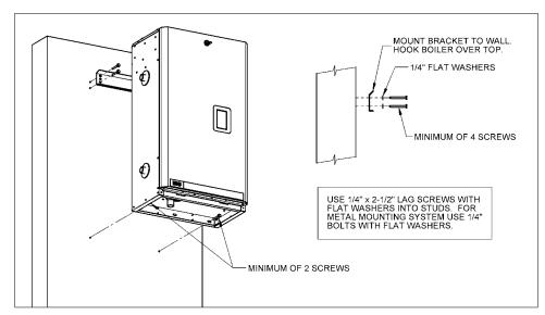
Figure 3: Wall mounting of boiler
