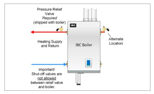
Figure 29: Relief piping with single side piping connections
