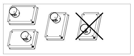
Figure 15: Allowed SST installation orientations
