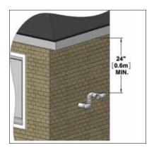
Figure 8: IBC recommended minimum vent terminal clearance under ventilated soffit
