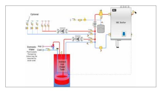
Figure 36: Indirect Domestic Hot Water piping concept
