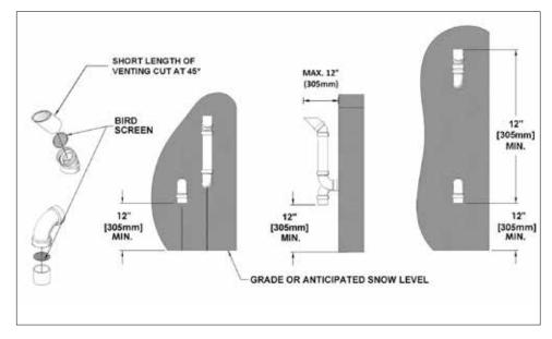
Figure 13: Sidewall vent termination - piping configuration
