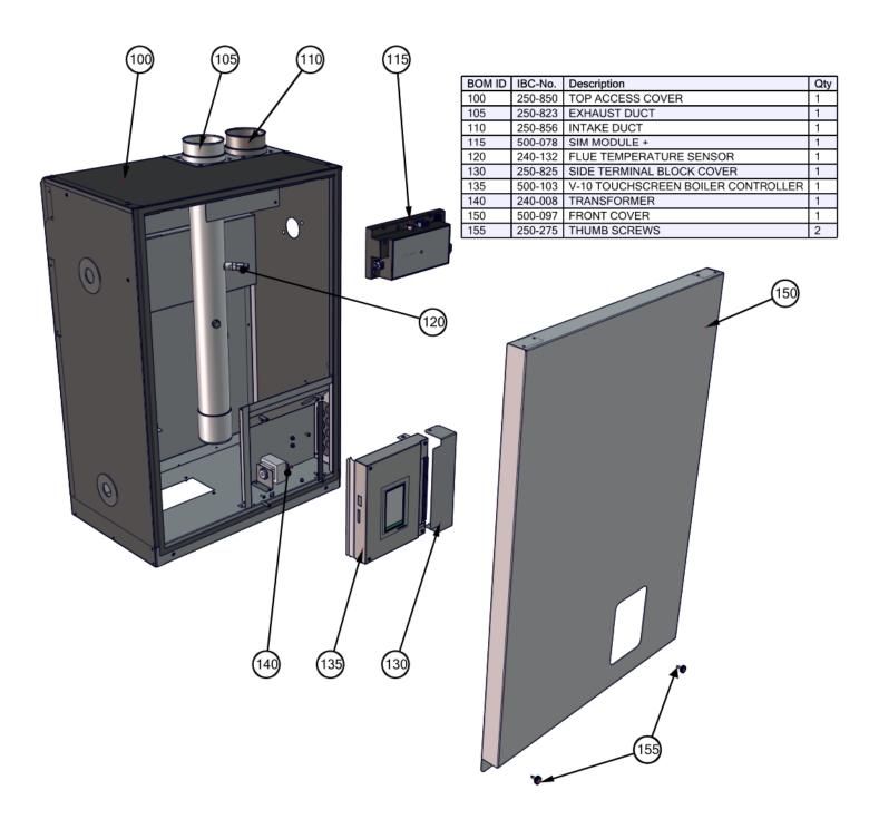
Diagram 6.1-2: Boiler assembly parts
