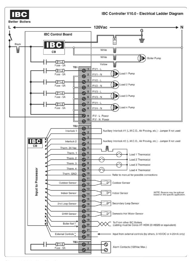
Diagram 6.2-1: Ladder wiring diagram
