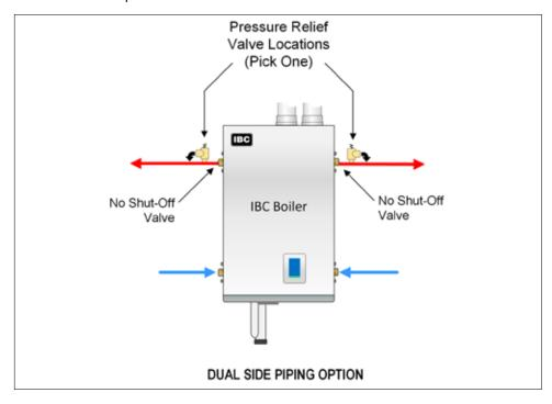
Figure 30: Relief piping with dual side connections
