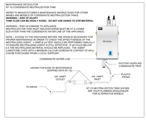
Figure 27: Condensate neutralization tank
