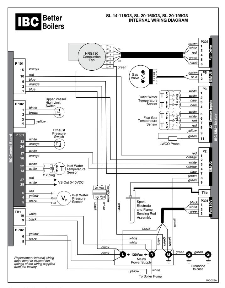
Diagram 6.2-2: Internal wiring diagram
