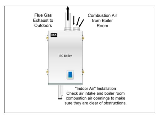
Figure 20: Indoor combustion air intake
