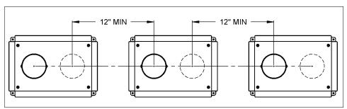
Figure 18: Minimum separations for multiple vent installation - horizontal orientation
