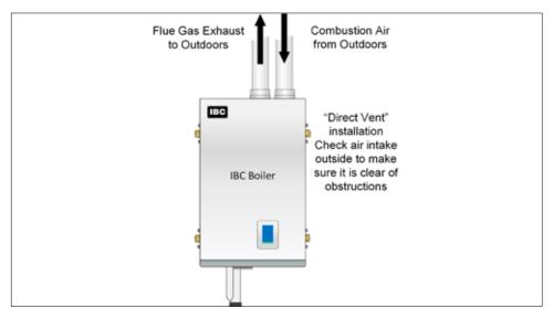
Figure 19: Direct vent combustion air intake
