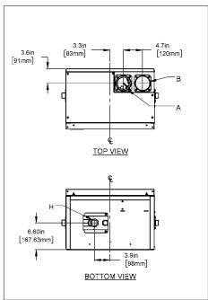
Figure 2: Dimensions / Connections for SL 20-160 G3 - Front view, side view, top view and bottom view
