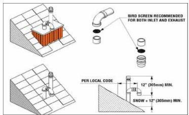
Figure 6: Rooftop vent terminal configurations
