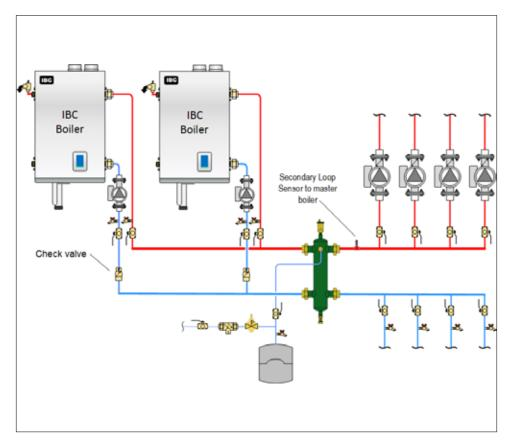
Figure 42: Multiple boiler low loss header piping concept
