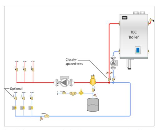
Figure 33: One-temperature space heating piping concept - tees on secondary piping
