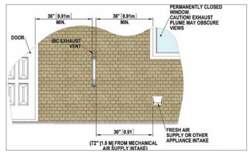
Figure 11: Vent terminal clearances
