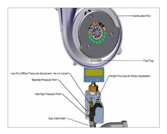
Figure 45: Gas Valve and Pressure Reference System
