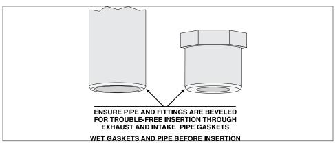
Figure 5: Pipe and fitting beveling
