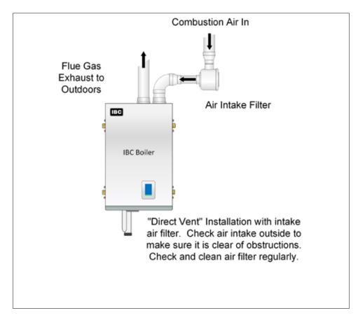
Figure 23: Direct vent - intake, exhaust system with optional air intake filter (filtration may also be used on indoor air applications as required)
