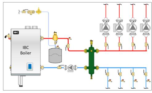
Figure 38: Basic Primary-Secondary piping with hydraulic separator concept
