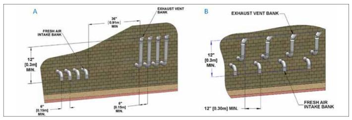
Figure 14: Sidewall vent termination - multiple vent piping configuration
