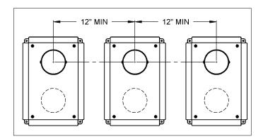
Figure 17: Minimum separation for multiple vent installation - vertical orientation
