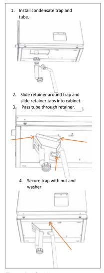
Figure 24: Condensate trap installation
