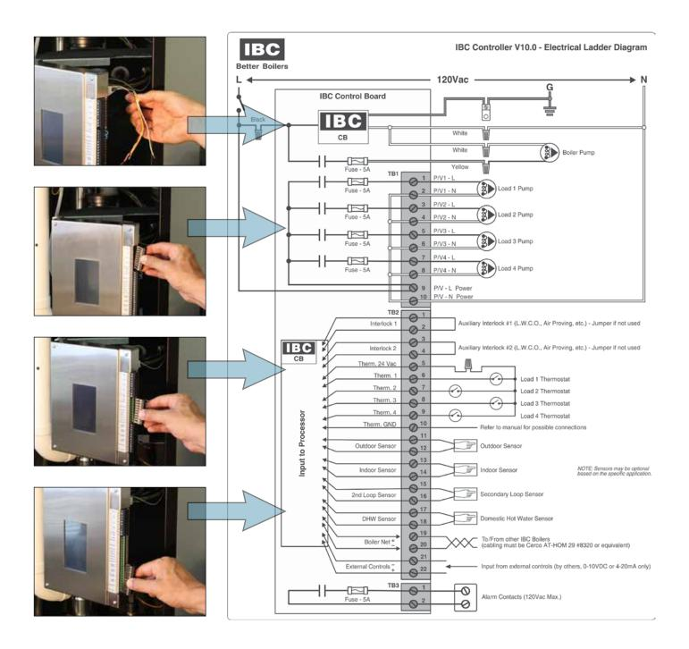
Figure 44: Electrical Wiring Connections (full page ladder diagram at back of this manual)
