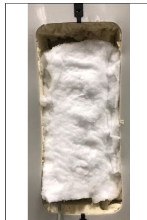
Figure 16 - Superwool Insulation Installed
