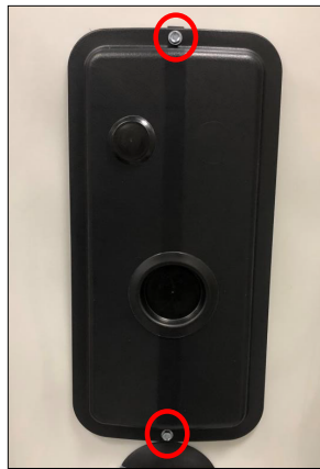
Figure 10 - Screws Securing the Access Panel
