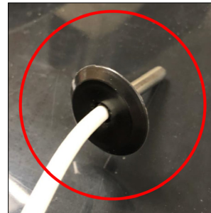
Figure 14 - Sensor Through the 3/4" Plug
