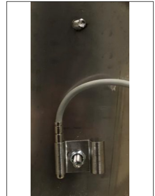
Figure 15 - Sensor Clip on the Lower Stud
