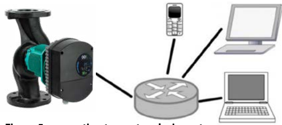
Figure 5: connecting to a network via router
