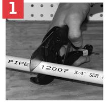
Acceptable tools include ratchet type pipe cutter,
