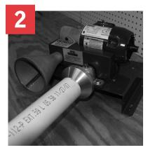
• Chamfer (bevel) the end of the pipe 10° - 15°.
