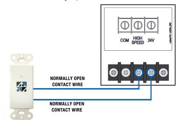
FIGURE 4.8.1 LOW VOLTAGE WIRING DIAGRAM 2
