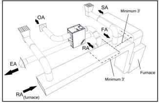
FIGURE 2.4.3 FURNACE RETURN AIR BACK INTO RETURN AIR
