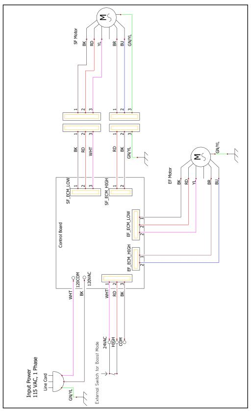
FIGURE 4.7.0 EV PREMIUM WIRING SCHEMATIC
