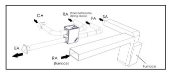
FIGURE 2.4.2 SEPARATE RETURN AIR AND FRESH AIR SUPPLY
