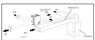
FIGURE 2.4.1 SEPARATE ROOM AIR PICK-UP—FRESH AIR TO FURNACE RETURN AIR TRUNKLINE
