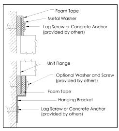
FIGURE 3.1.0 MOUNTING THE ERV TO A STUD WALL
