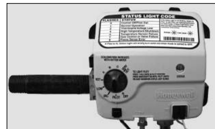
Figure 56 - Gas control/valve with threaded pipe.
