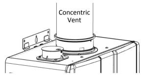
Secure the vent pipe to the concentric flue connection with the supplied screw.
