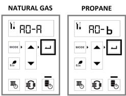
7. Parameter settings are complete. To enter normal operation mode, press the **Mode** button.
