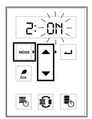
Press the **Mode** button twice. **2:0N** should appear on the display. Press the **Up** or **Down** arrows to select ON or OFF.
