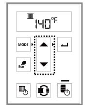
Adjust the temperature with the **Up** or **Down** arrows until the appropriate temperature is displayed.
