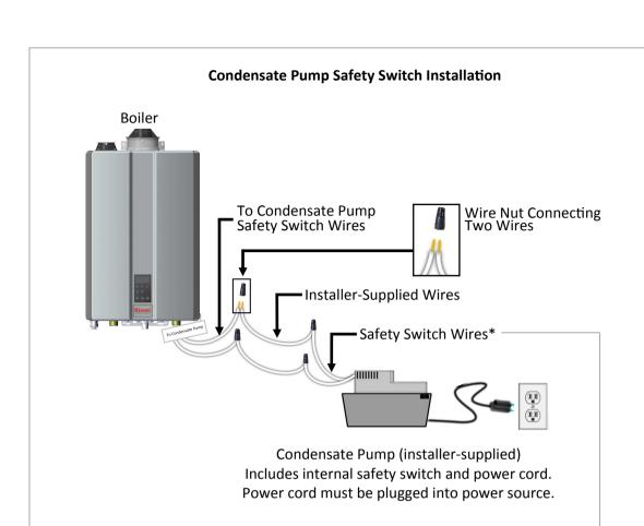
\* Safety switch wires connect to the NO and COM contacts on the safety switch.
