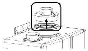
Install the concentric vent. Ensure it is properly seated.
