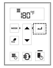
Press the **Select** button to confirm the temperature.
