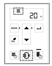
Press the **Switch Operation Mode** button until the **Central Heating Active** button appears on the home screen.
