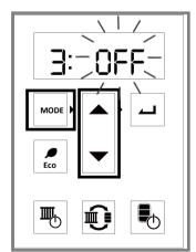
Press the **Mode** button three times. 3: OFF should appear on the display. Press the Up or Down arrows to select:
