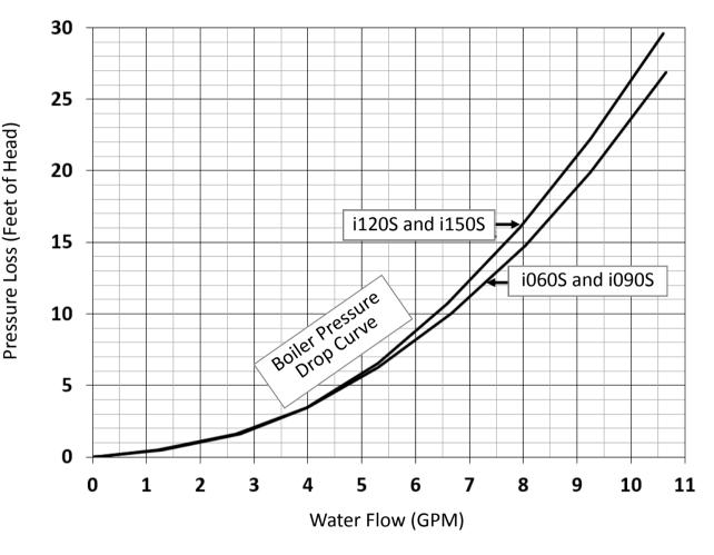
Below are options for the primary pump circulating across the boiler. No additional pressure drop is accounted for through the system piping or system components. Recommended circulation pumps are listed below. The maximum amperage permitted is 2 Amps.
