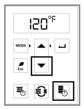
While continuing to hold the ▼ (Down) button, press and hold the **Indirect Tank** button (press and hold both buttons down at the same time).
