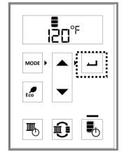
Press the **Select** button to confirm the temperature. The setpoint temperature displays for a few seconds and then returns to standby mode.
