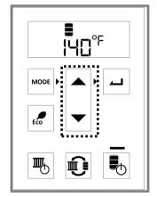
Adjust the temperature with the **Up** or **Down** arrows until the appropriate temperature is displayed.
