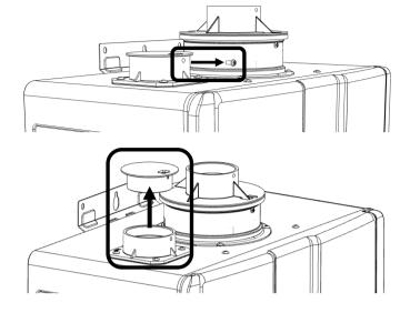
Install the combustion air vent pipe. Ensure it is properly seated.
