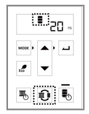
Press the **Switch Operation Mode** button until the **Indirect Tank** icon appears on the home screen.
