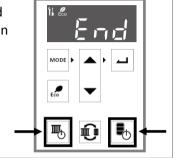
2. On the PC Board, press and hold the top, left black button shown below. The **Maintenance Required** icon (see right image) on the controller display will appear.
