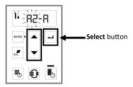
7. Press the ▲ (Up) or ▼ (Down) arrows until ☐ □ b appears in the display. Then, press the Select button.
