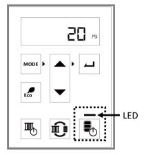
If the LED above the **Indirect Tank** button is not illuminated, press the **Indirect Tank** button.
