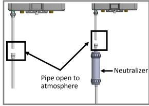
Refer to neutralizer Installation Manual and local codes for neutralizer installation guidelines.
