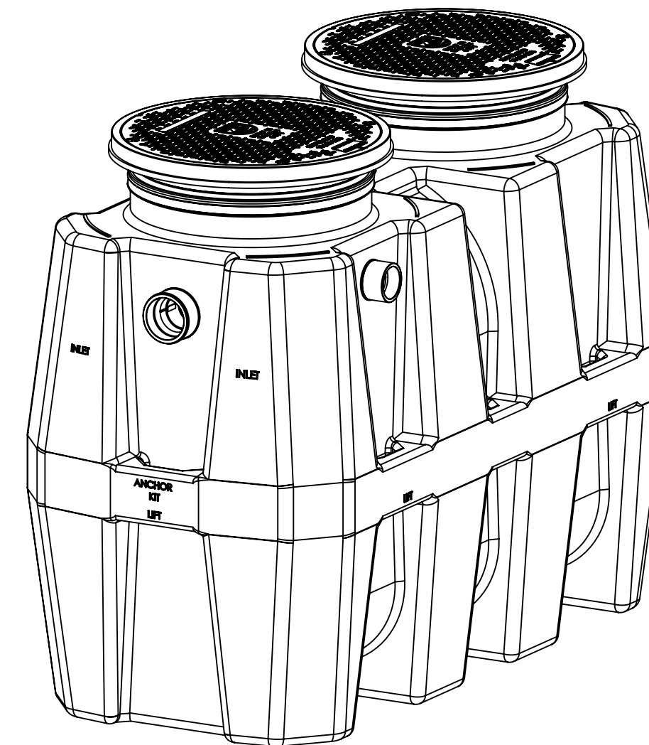
OS-100 100 gpm, 250 gallons 144 gallon oil capacity 95 gallon sand capacity
