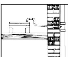
**CONNECTION TO DRAIN STACK PIPE**
