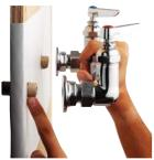
Step 1: Apply plumber's putty to backside of body and insert into mounting hole. Line up water supply lines and couplings, attach and tighten with
