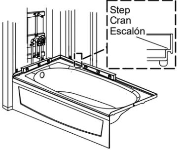
**9** Secure the metal support clips to the studs. Bend the tabs over the flange.
