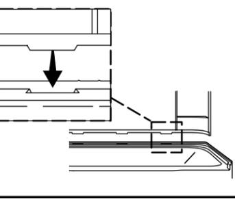
**15** Measure, mark, and drill the faucet holes in the end wall.
