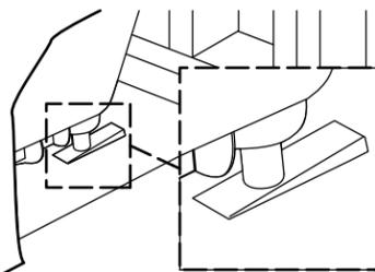
**12** Connect the bath drain to the drain pipe. Position a protective liner in the bath.
