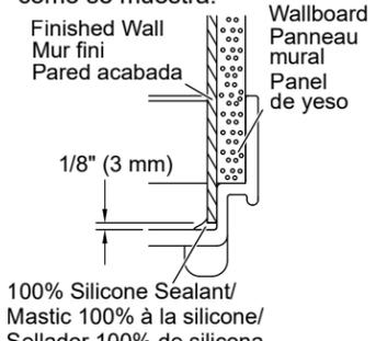
**14 STERLING Wall Set:** Install the back wall. Insert the tabs into the slots.
