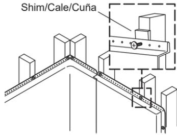
**21** Cover the framing with water-resistant wallboard. Install the finished wall material.
