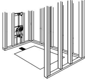
**5** Without a pad, set the basin area in 1" (25 mm) to 2" (51 mm) of mortar cement.
