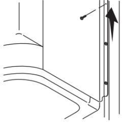
**20** Secure the walls to the studs along the top. Use shims as needed.
