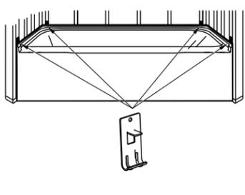
**8** Level the unit using the step of the flange.
