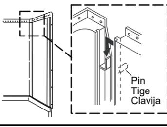
**18** The front edges should be flush, with no more than a 1/32" (1 mm) gap.
