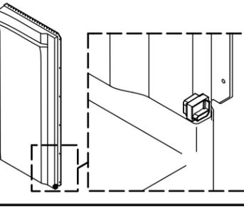
**17** Install the end walls. Engage the pins in the slots.
