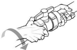
**STEP 9** Pressure test the system only after all solvent cement joints have fully cured. If any leaks are found at End Connectors during pressure check, use a strap wrench to tighten Union Nut 1/4 turn to stop the leak.
