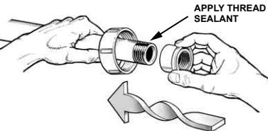
**STEP 3** Wrench Make Up - Threaded pipe and valve components must always be installed using commercially available strap wrenches. Do not use conventional pipe wrenches, which can cause damage to plastic piping materials. Apply wrench make-up of no more than 1 to 2 turns beyond finger-tight thread engagement. Care must be taken in final positioning so as to avoid the need to "Back-up" the wrench assembly.
