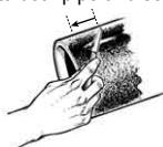
Check the penetration and softening by scraping the primed surfaces. A few thousandths of the semi-fluid surface should easily be removed.
