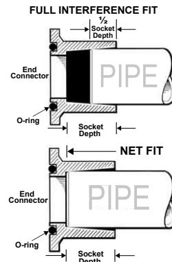
**STEP 3** Check the Joint Interference fit between the pipe and the End Connector Socket. An Interference Fit is necessary for proper fusion of the joint. To check, lightly insert the End Connector Socket over the prepared pipe ends. DO NOT FORCE THE SOCKET ONTO THE PIPE.
