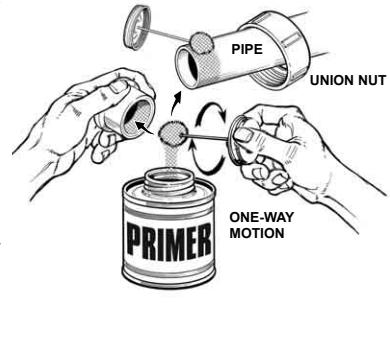
Using a brush or applicator size no less than 1/2 the pipe diameter, apply a liberal coat of primer with a circular, scrubbing motion to the inside socket of the End Connector until the surface is softened and semi-fluid. This will occur in 5 to 15 seconds, depending on size and temperature.
