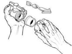
**STEP 2** Remove Union Nuts (1) and End Connectors (2) from the Valve Body (3). Wipe away all loose dirt & moisture from the pipes & components with a clean dry cloth. Slide Union Nuts (1) over pipe ends where each End Connector Socket is to be installed, being sure that the Union Nut threads will be facing the Valve body.
