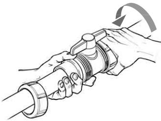
BE SURE THAT THE FACE OF THE END CONNECTOR SOCKET IS SQUARELY ALIGNED (FLUSH) WITH THE VALVE BODY AND IS FLUSH AGAINST THE O-RING.
