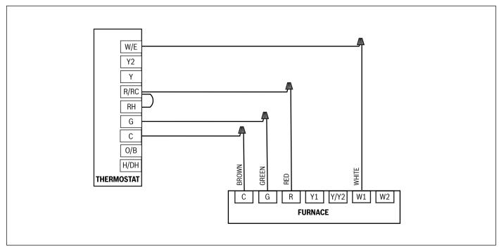
Figure 52 Wiring Detail - Furnace and Bosch Connected Control BCC50
