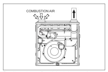
Figure 42 Combustion Airflow Path Through The Furnace Cabinet
