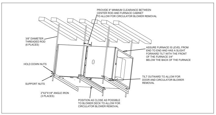
Figure 10 Horizontal installation
