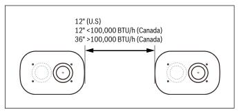
Figure 33 Multiple flush mount vent terminations clearance
