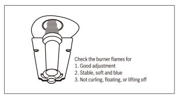
Figure 57 Burner Flame
