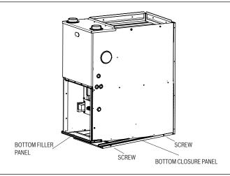
Figure 7 Removing bottom closure panel
