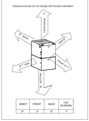
Figure 3 Minimum clearance from combustible construction
