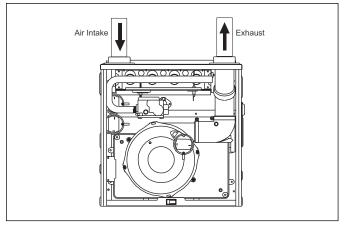
Figure 41 Direct vent air intake connection and vent connection
