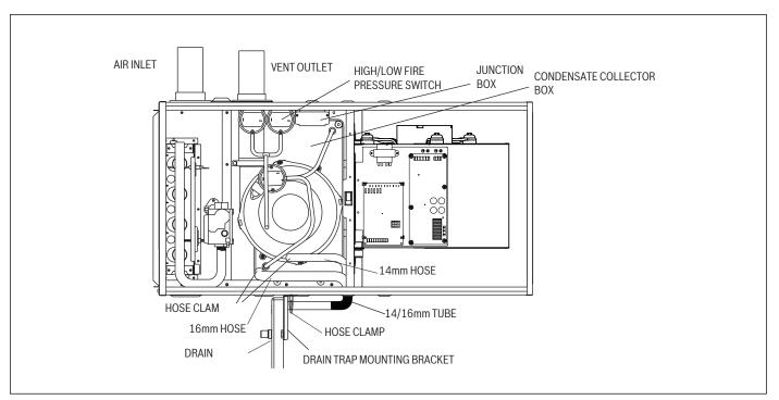
Figure 21 Horizontal left side installation, vent through side panel
