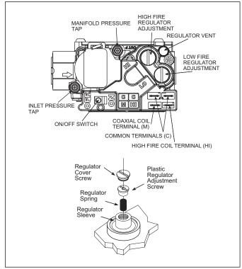
Figure 55 Gas valve and regulator adjustment
