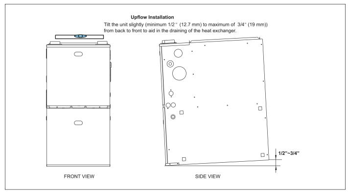
Figure 8 Upflow application-setting equipment
