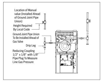
Figure 45 Typical Gas Pipe Arrangement
