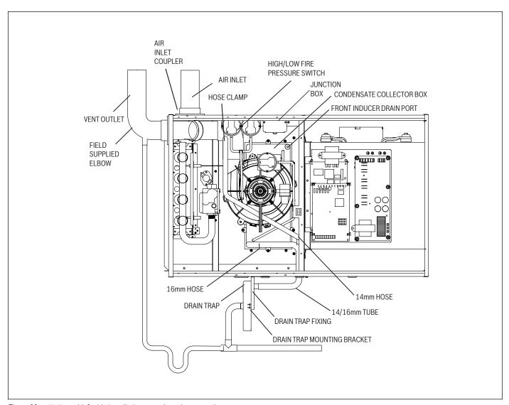
Figure 20 Horizontal left side installation, vent through top panel
