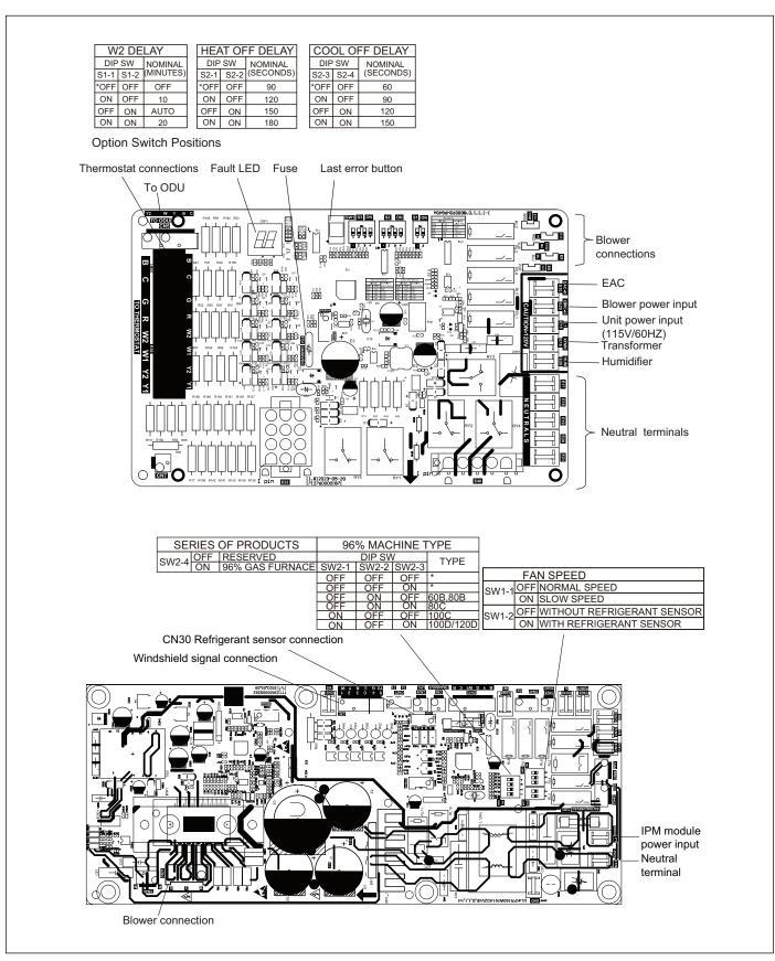
Figure 47 Furnace Control
