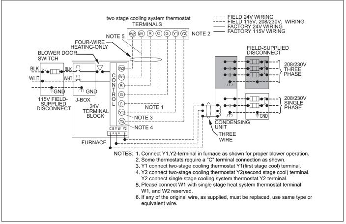
Figure 48 Heating and Cooling Application Wiring Diagram with 2-Stage Thermostat
