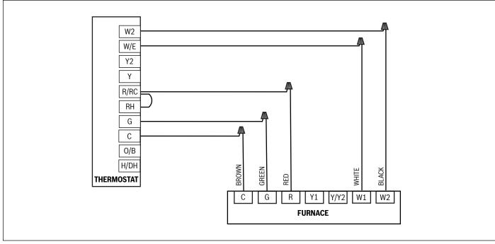
Figure 51 Wiring Detail - Furnace and Bosch Connected Control BCC100
