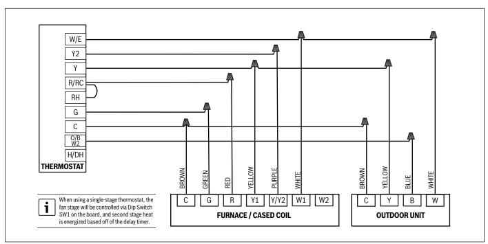
Figure 54 Wiring Detail - Furnace/Cased Coil, Bosch IDS Outdoor Unit and Bosch Connected Control BCC50
