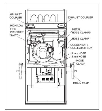
Figure 15 Upflow installation, top venting
