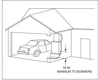
Figure 6 Installation in a garage
