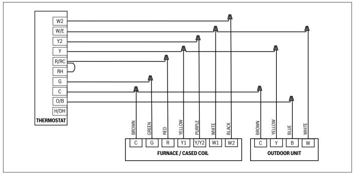
Figure 53 Wiring Detail - Furnace/Cased Coil, Bosch IDS Outdoor Unit and Bosch Connected Control BCC100
