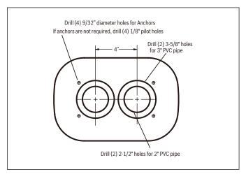
Figure 37 Mounting template
