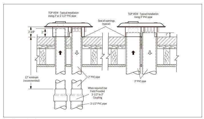
Figure 39 Typical installation
