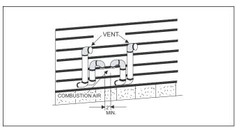
Figure 30 Double horizontal combustion air intake and vent termination
