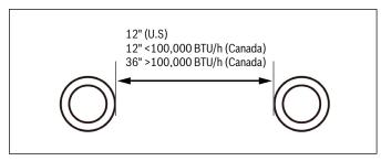
Figure 32 Multiple concentric vent terminations clearance
