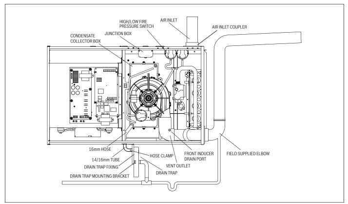
Figure 17 Horizontal right-hand side installation
