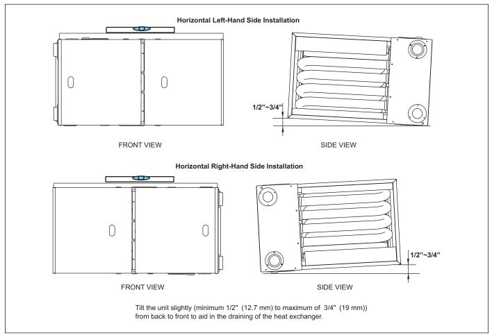
Figure 9 Horizontal application-setting equipment
