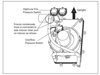
Figure 19 Pressure switch position
