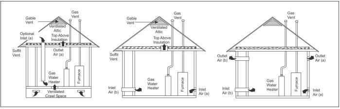
Figure 43 Ambient Combustion Air
