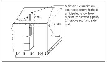
Figure 27 Termination configuration - 1 pipe
