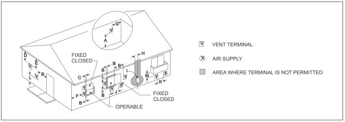
Figure 26 Direct vent terminal clearances
