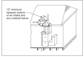
Figure 44 Attic and Crawl Space Combustion Air Termination
