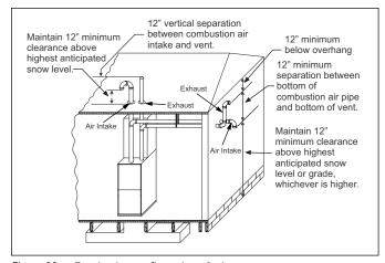
Figure 28 Termination configuration - 2 pipe
