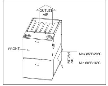
Figure 5 Return air temperature
