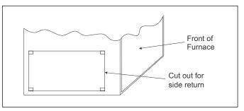
Figure 23 Side return knockout markings
