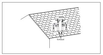
Figure 31 Double vertical combustion air intake and vent termination
