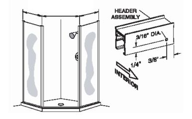
Press the header assembly [**D**] over the wall jambs [**E**] and 135° posts [**K**]. Check the posts for plumb. Adjust as required by varying the overlap of the header over the wall jambs. You may need to trim the ends of the header where it meets the wall. The minimum horizontal dimension for the door opening is the door panel width (see the graphic in Step #9) plus 1/2", maximum is the door panel width plus 1 3/4".
