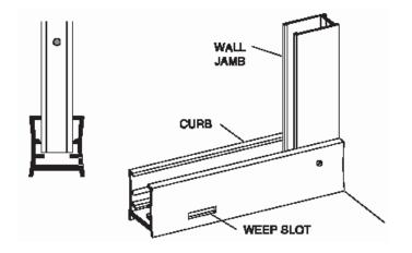
Wipe the shower walls and sill, curb assembly [A] and wall jambs [E] with a clean, dry cloth to remove any dust or debris. Apply a 1/4" bead of caulk along the inside of both of the pencil lines marked in Step #3. Carefully replace the curb in the exact position marked. Caulk the inside of the curb ends where they meet the wall. Caulk around the anchor plates [B], screws [C], and the insides of the mitered joints.
