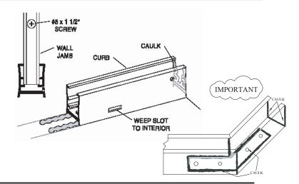
Place the setting blocks [H] in the curb mbly [A] as shown to support the two fixed glass panels [J]. The setting blocks should be positioned approximately 3" from each corner of the panels. Remove any protective strips from the first glass panel and set it into place. It should rest on the setting blocks and be engaged approximately 1/2" into the wall jamb [E]. A strip of masking tape 1/2" from each vertical edge of the glass will aid alignment.
