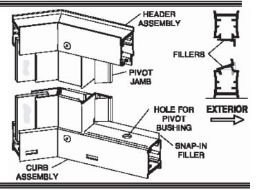
Pull the bottom end of the pivot jamb [N] tight to the curb filler [R] and plumb the jamb. Drill two 1/8" holes thru the pivot jamb and into the 135° post [K] in line with the screws in the head and curb and approximately 1/4" vertically from the ends of the jamb. Drill a third hole centered between the first two, then enlarge the outer holes with a 3/16" drill for clearance on the self-tapping screws. Attach the pivot jamb permanently with three #8 x 1/4" truss head screws [C].
