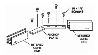
The curb should sit near the centerline of the sill. If required, use a file to round the lower ends of the curb assembly to fit the shower sill properly.
