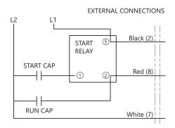
Figure 1. Wiring Diagram 1-Phase, External Capacitor
