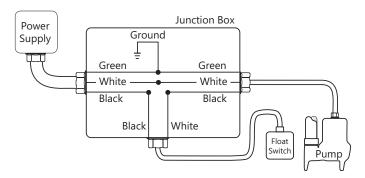
Figure 3. Direct Wiring of 208/230V, 1-Phase, Automatic Pumps
