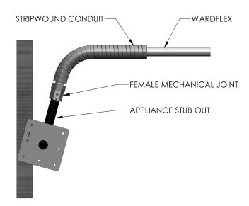
Figure 4.4 Appliance stub out with a WARDFlex®/WARDFlex®MAX female mechanical fitting which can be installed in a concealed location. For this type of arrangement refer to section 4.4 on for protection details.
