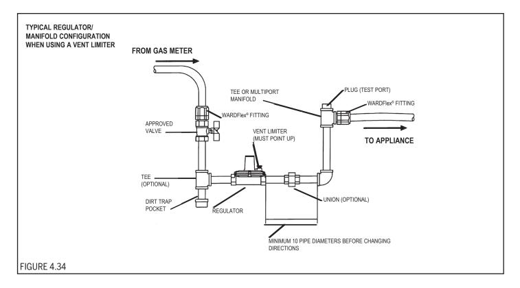
Regulators used to reduce elevated system pressure for appliance use must also conform to the following:
