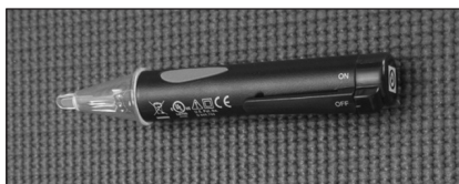
Figure 33 - Use a non-contact circuit tester to check for electrical power.
