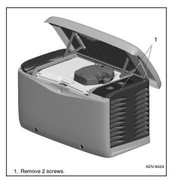
Figure 1-4 Removing the Air Intake Panel
