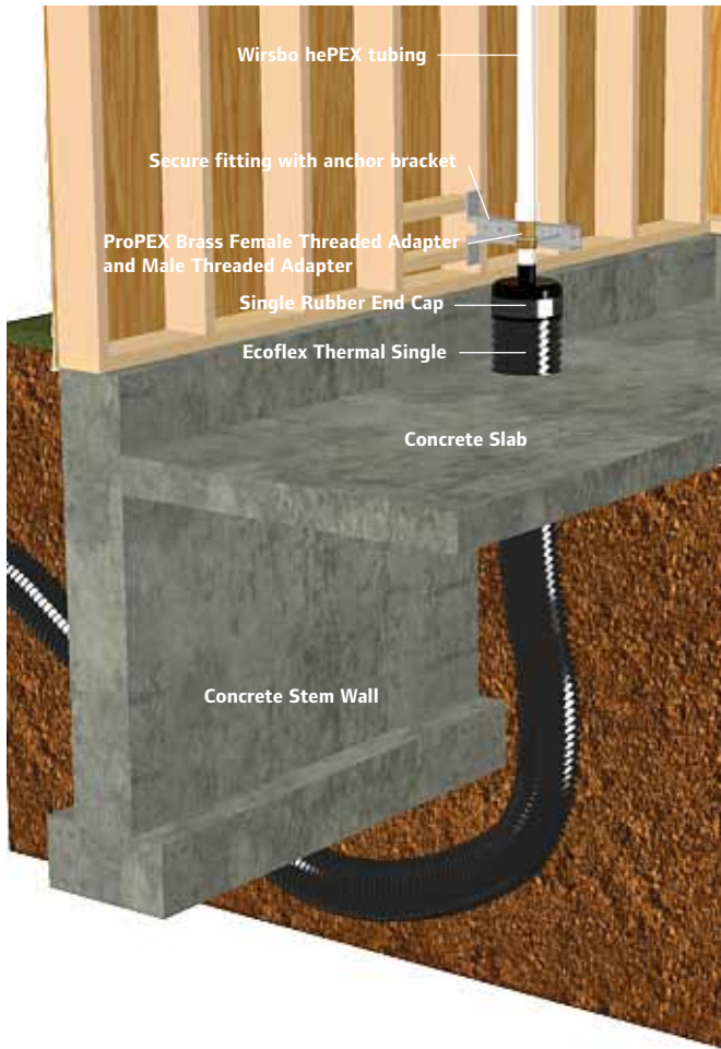
Figure 44: Slab-on-grade Under Footing Installation – Interior Wall Attachment
