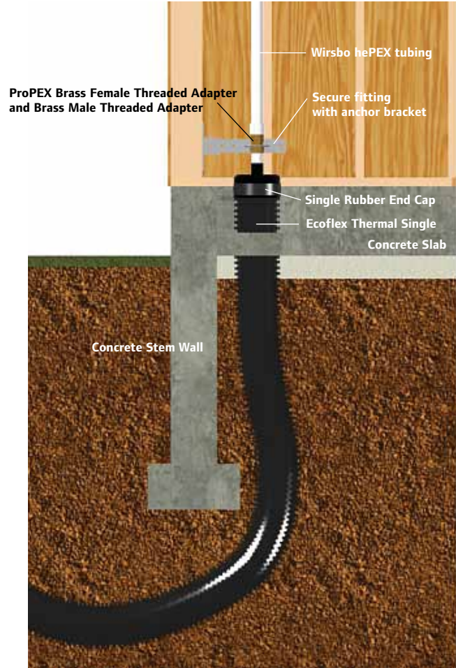
Figure 45: Slab-on-grade Under Footing Installation –Interior Wall Attachment
