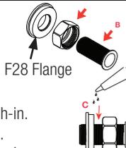
Loctite must cure for 24 hours before turning on water; otherwise the Loctite will wash out and joint will leak.
