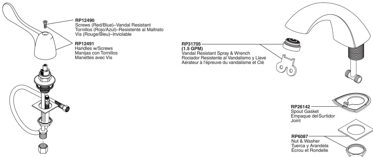
1. Apply plumber tape to male threads on hoses.
