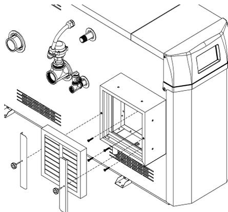
**2** Secure filter kit using factory screws removed in step 1. Reuse the factory gasket.
