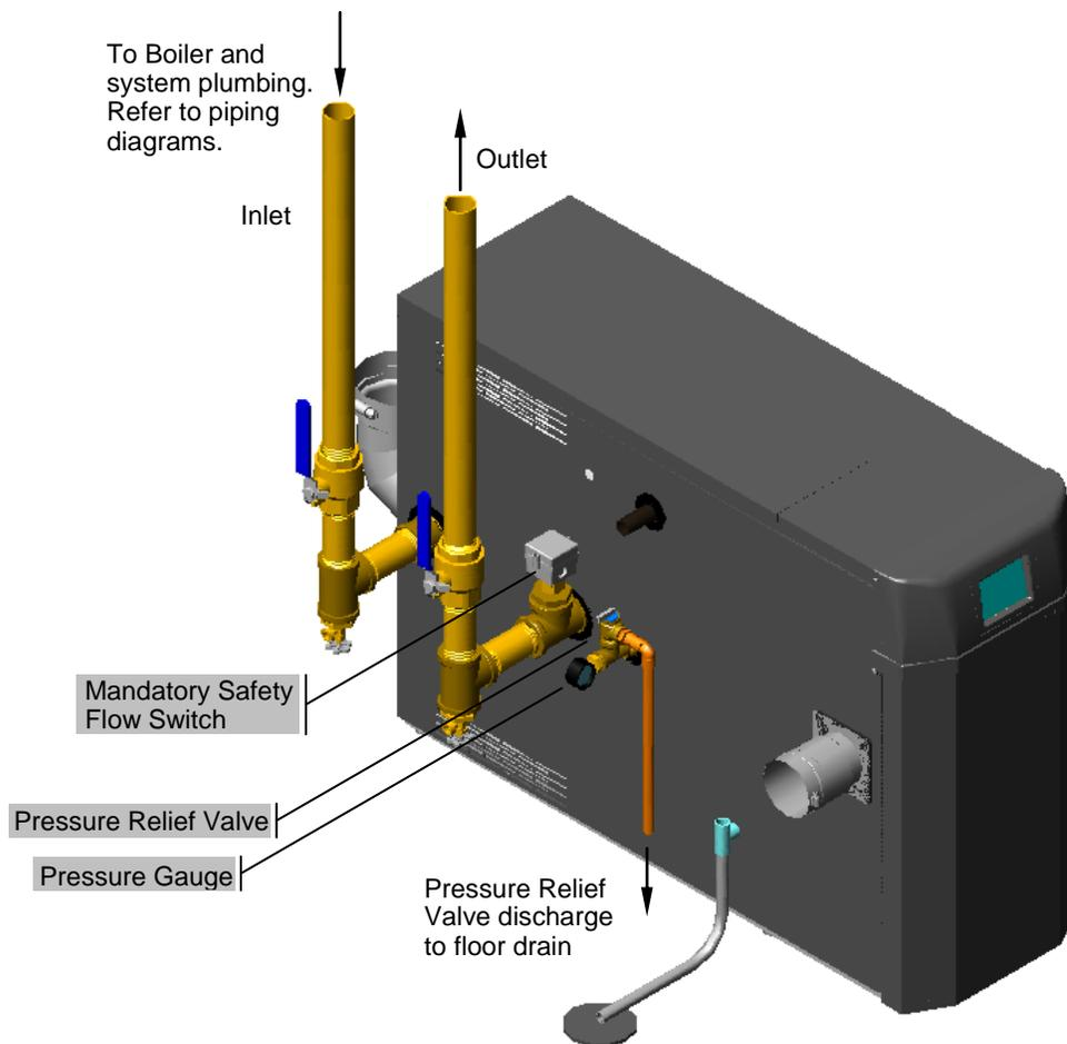
**Low Water Cutoff (LWCO) / Safety Flow Switch** – Trinity Lx150-400 boilers are provided with a factory installed Water Pressure Switch; in the event the pressure drops below 10 psi, the burner is inhibited from firing. Where required by the Authority having jurisdiction, an external LWCO, or Safety Flow Switch, may have to be installed; see Figures 10-1(a) and (b) for Safety Flow Switch installation.
