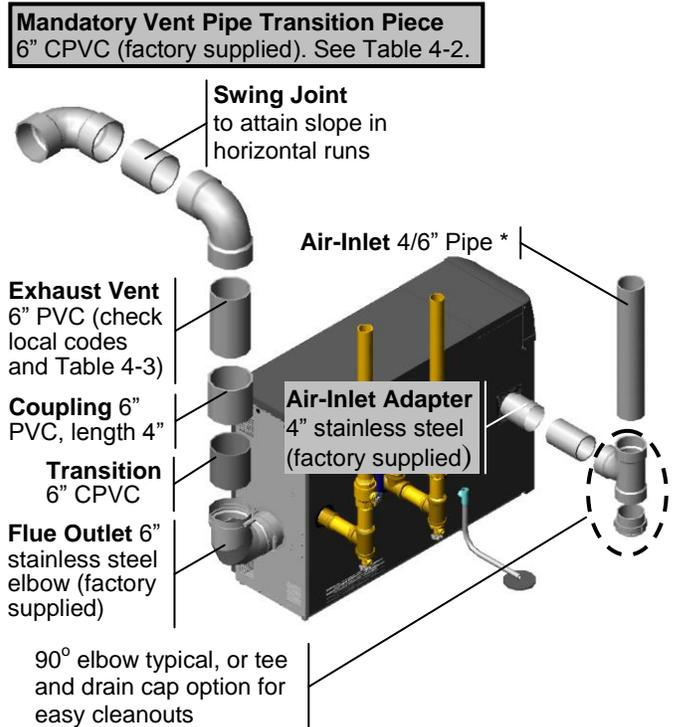
\* **Air-Inlet** - check with applicable local codes for acceptable pipe material.
