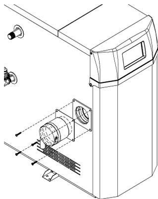
**1** Remove factory appliance air-inlet adapter; keep screws from installation of filter kit
