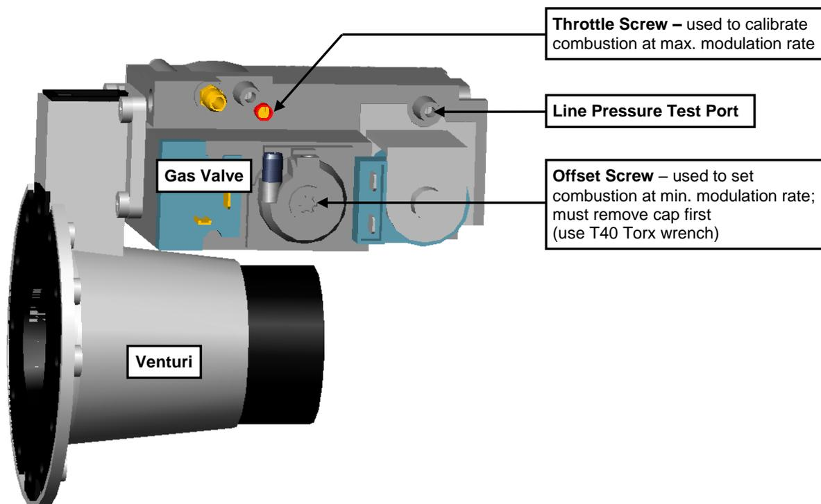
Figure 9-3 Gas Valve Assembly (Lx500)
