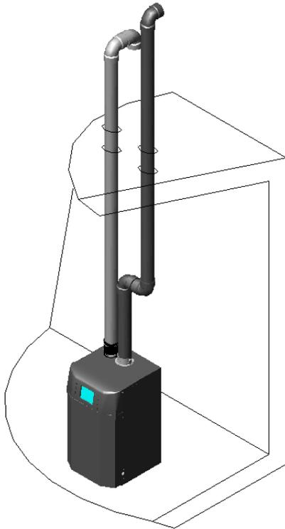
**Figure 4-8(b) Concentric Roof Termination**
