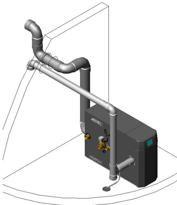
**Figure 4-7(b) Two-Pipe Sidewall Termination**
