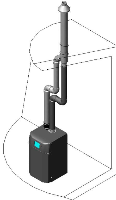
Sidewall Termination Details – Direct Vent Installation
