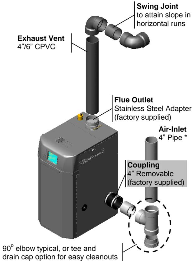
Figure 4-3(b) Lx300-400 Near Boiler Venting (PVC)
