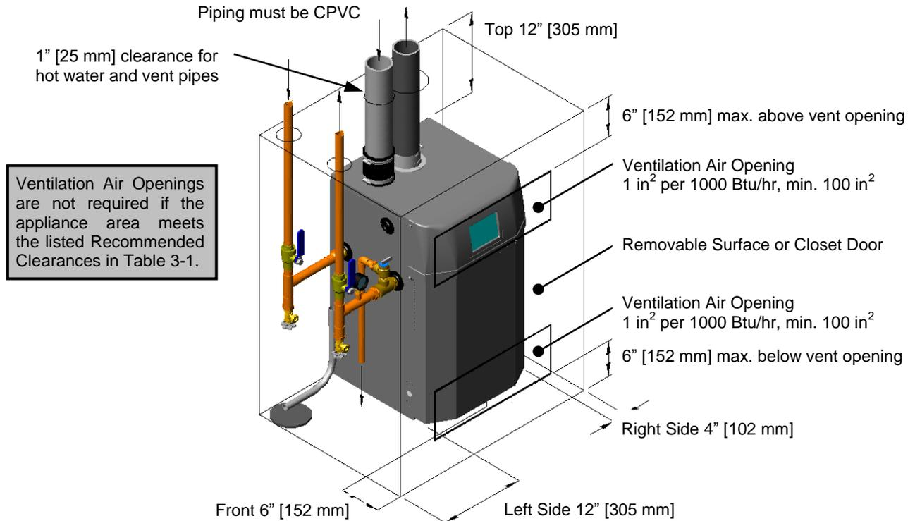
Figure 3-1(b) Closet Installation, Minimum Clearances (Lx300-400)
