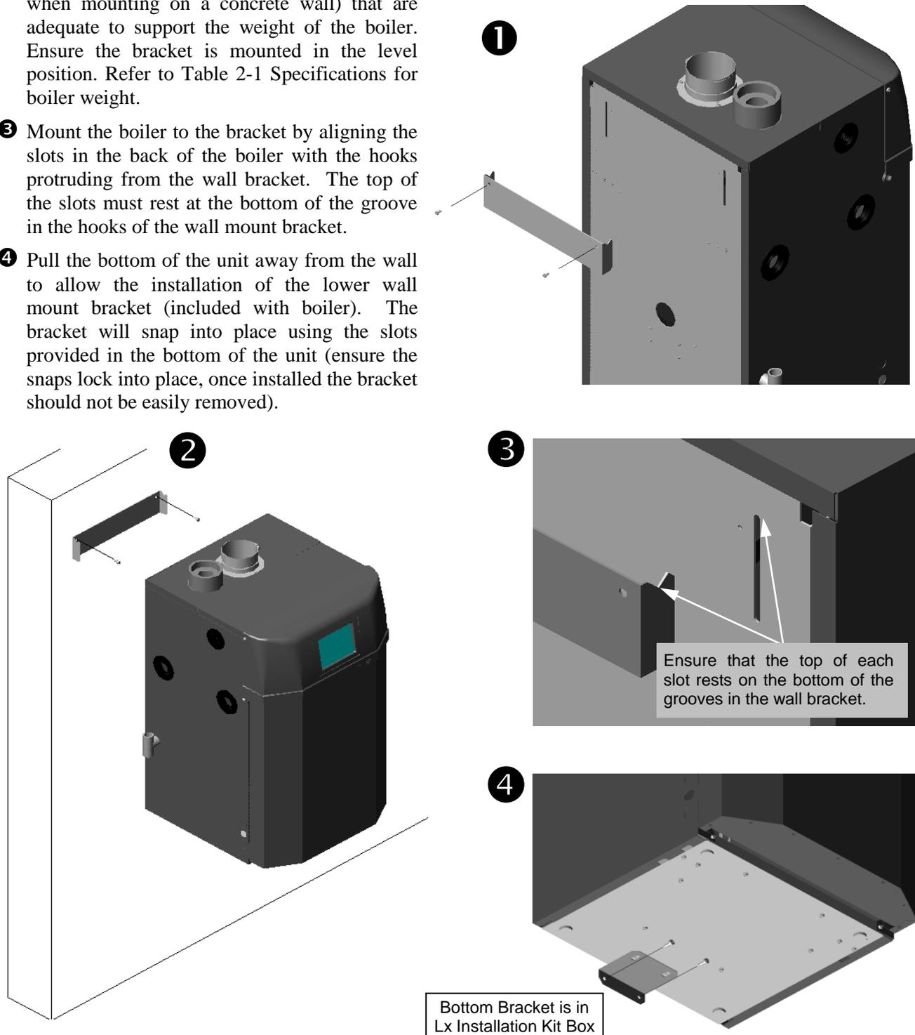
Figure 3-2(b) Wall Mounting Installations (Lx300-400)
