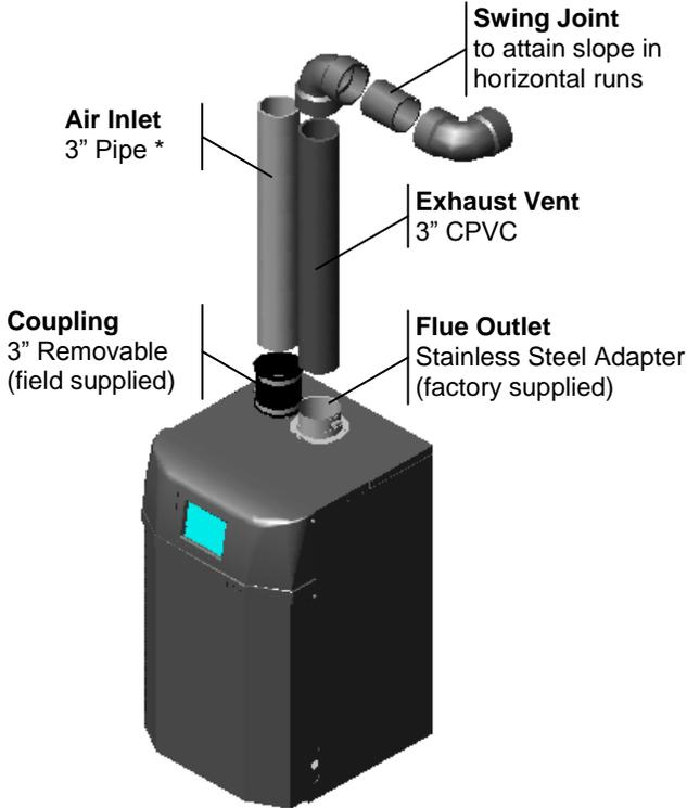
Figure 4-2(b) Lx150-200 Near Boiler Venting (PVC)
