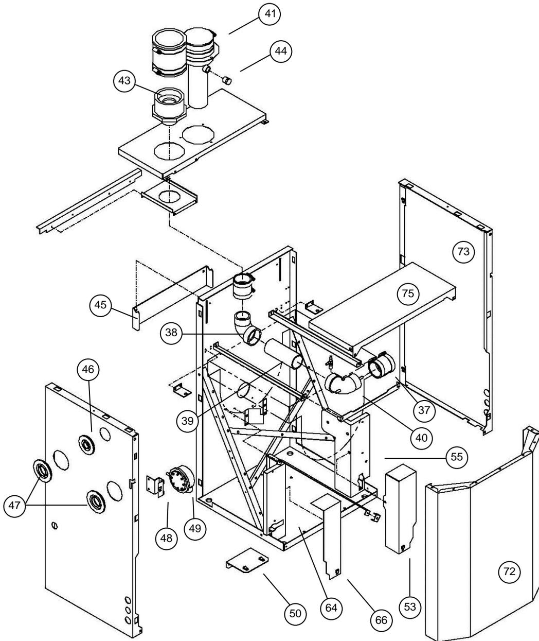
Figure 16-2 Heat Exchanger, Gas Valve, Blower and Burner Assembly (Lx150-200)
