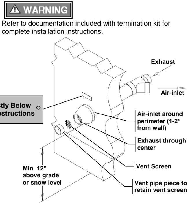
Figure 4-9(c) Low Profile Termination (Sidewall)      Figure 4-9(d) PolyPro / InnoFlue Termination (Sidewall)
