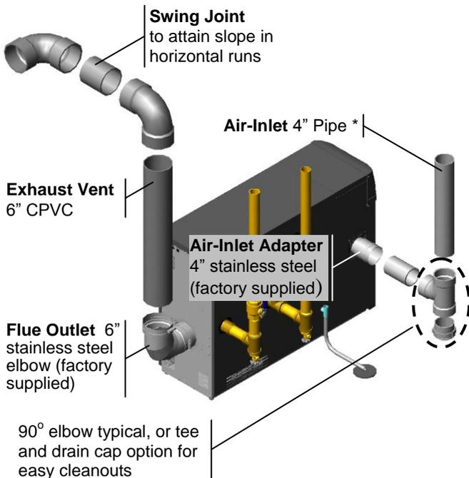
Figure 4-5(b) Lx700-800 Near Boiler Venting (PVC)
