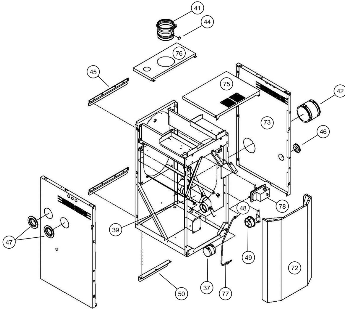
Figure 16-5 Heat Exchanger, Gas Valve, Blower and Burner Assembly (Lx300-400)
