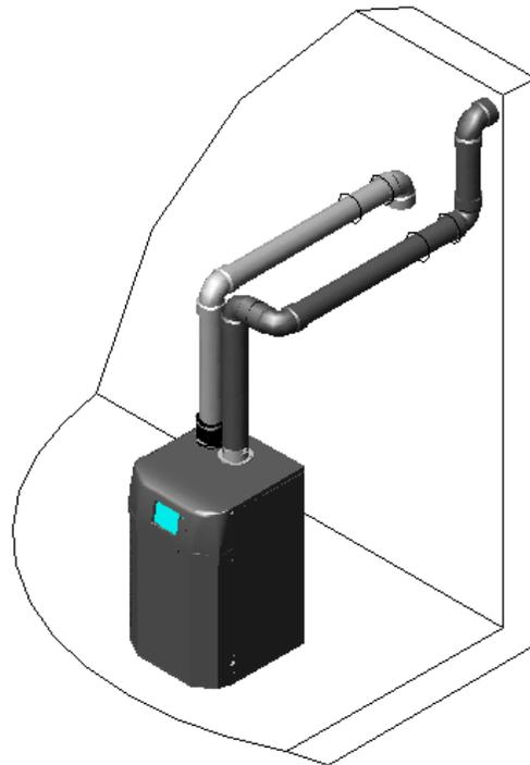
**Figure 4-7(a) Two-Pipe Sidewall Termination**
