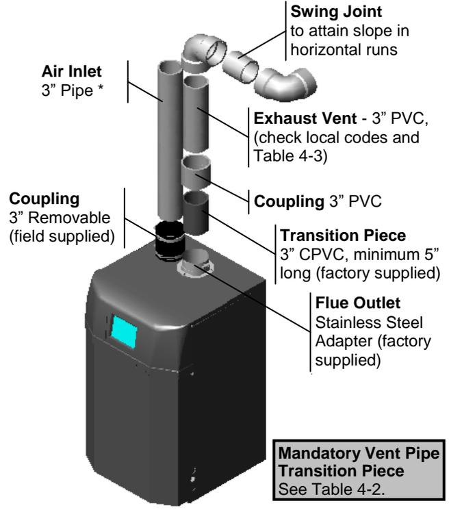
Figure 4-3(a) Lx300-400 Near Boiler Venting (CPVC)
