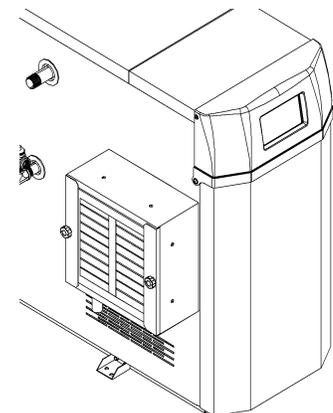
**3** Secure the filter in place with the brackets and knurled screws provided in the filter kit.
