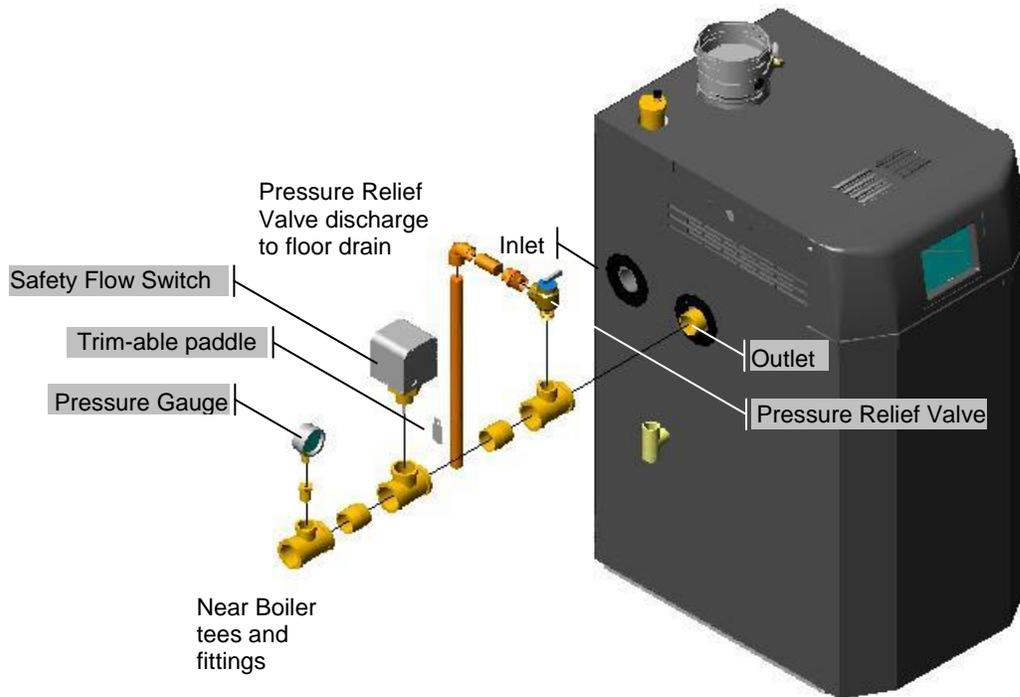
Figure 10-1(b) Near Boiler Piping (Lx500-800)
