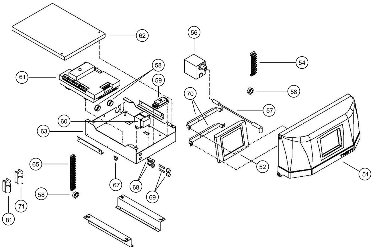
Figure 16-4 Cabinet, Vent and Air-Intake Parts (Lx300-400)
