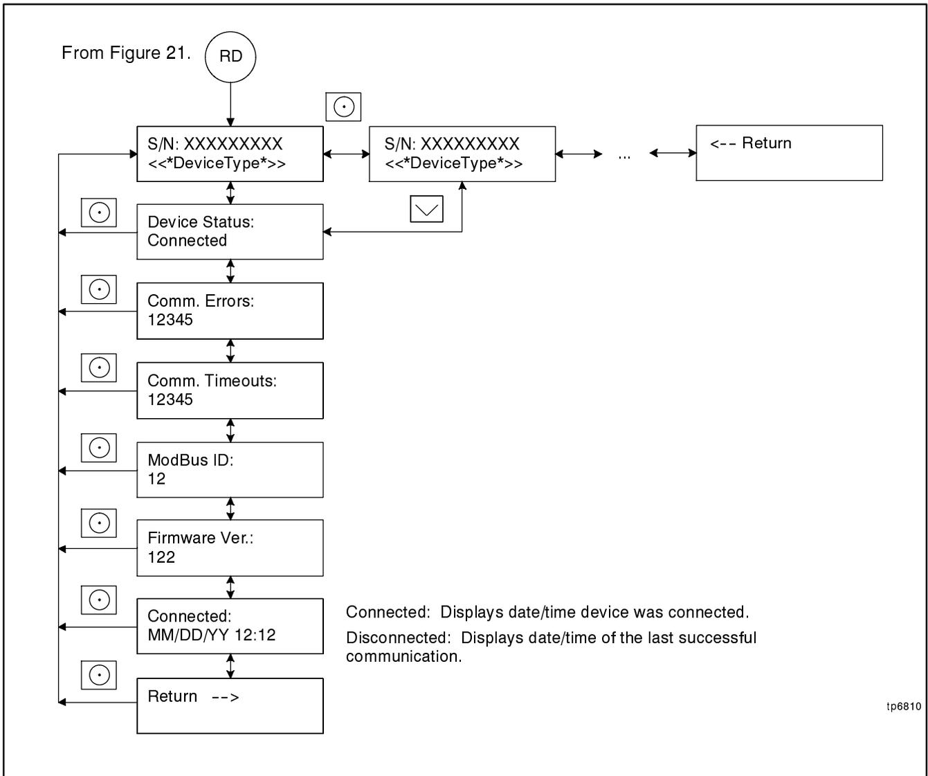
**Figure 22** RDC2 Controller, Remote Devices Submenu
