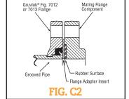
NOTE: The Gruvlok Fig. 7012 Flange requires the use of a Flange Adapter Insert when used against rubber surfaces (Figure C1), serrated flange surfaces or mating flanges with inserts (Figure C2). The Flange Adapter Insert will be exposed to the fluids in the system. Ensure that the Insert is compatible with the fluids in the systems and with adjacent piping components.
