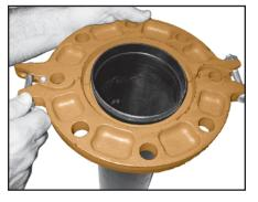
$\label{eq:lastice} \begin{array}{c} \textbf{2} \textbf{LATCH HOUSINGS} \\ \textbf{-} \textbf{Place the latch} \\ \textbf{bolt back into the slotted hole. Tighten the} \\ \textbf{nut until there is a $\frac{1}{16}$" gap between the flange halves at location "A". (See Figure below) \\ \end{array}$
