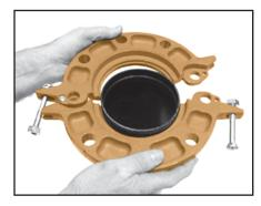
**1 INSTALL HOUSINGS**—On the side without the hinge pin, loosen the latch bolt nut to the end of the bolt thread. (It is not necessary to remove the nut from the latch bolt.) Swing the latch bolt out of the slot. Open the Gruvlok Flange and place around the grooved pipe end with the key section fitting into the groove. The flange gasket cavity must face the pipe end.
