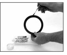
**3**CHECK & LUBRICATE GASKET— Check the gasket to assure that it is properly suited for the intended service. Lubricate the entire exterior surface of the gasket, including the sealing lips, using the proper Gruvlok lubricant.
