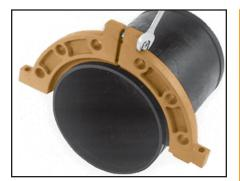
**INSTALL HOUSING**—Place each Gruvlok Flange segment around the grooved pipe with the key section fitting into the groove and the flange gasket cavity facing the pipe end. Loosely assemble the segments using the four segment-bolts-and nuts. Alternately and equally tighten the latch bolts and nuts to the specified latch bolt torque. Bring the four flange segments into full, firm metal-to-metal contact.
