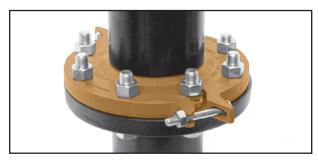
**INSTALL BOLTING**—Insert a flange bolt or stud with material properties of SAE J429 Grade 5 or higher through the bolt holes and thread a nut on hand tight. Continue this procedure until all bolt holes have been fitted. Tighten the nuts alternately and evenly so the flange faces remain parallel. All the bolts or studs must be torqued to the mating flange bolts specified torque. The flange faces should have metal-to-metal contact.
