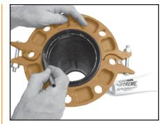
LUBRICATE GASKET LIP-With the gasket in place apply lubricant to the exposed gasket tip, which will seal on the mating flange. Tighten the nuts on the latch bolts alternately to the specified latch bolt torque. The flange housings must be in firm metal-to-metal contact.
