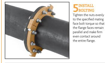
CAUTION: Proper torquing of flange bolts is required to obtain specified performance. Over torquing the bolts may result in damage to the bolt and/or casting which could result in pipe joint separation. Under torquing the bolts may result in lower pressure retention capabilities, lower bend load capabilities, joint leakage and pipe joint separation. Pipe joint separation may result in significant property damage and serious injury.
