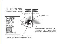
**GASKET POSITION**—The correct position and relationship of the components of the Gruvlok Flange assembly is shown in the Figure above. The wide gasket lip must seal on the pipe surface diameter and the narrow gasket lip must face the mating flange. Be careful that foreign particles do not adhere to lubricated surfaces.
