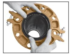
**INSTALL GASKET**—Stretch the Gruvlok gasket around the pipe end and then press the gasket into the cavity between the pipe O.D. and the flange. The gasket must be properly positioned as shown in the figure below.
