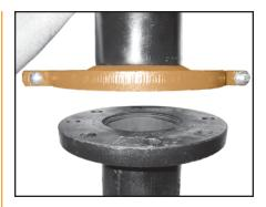
**INSPECT MATING FLANGE**—Verify Uthat the mating flange face is hard, flat and smooth, free of indentations, which would prevent proper sealing of the Gruvlok Flange gasket. Assure the gasket is still in the proper position and align Gruvlok Flange bolt holes with the mating flange, pump, tank, etc., bolt holes.
