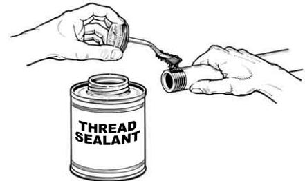
**STEP 1** Apply Joint Sealant - Threaded connections require application of a quality grade thread sealant to seal and lubricate the joint assembly. Sealants must only be applied to male pipe threads.
