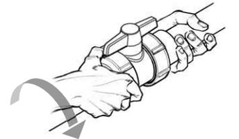
**STEP 9** Pressure test the system only after all solvent cement joints have fully cured. If any leaks are found at End Connectors during pressure check, use a strap wrench to tighten Union Nut 1/4 turn to stop the leak.
