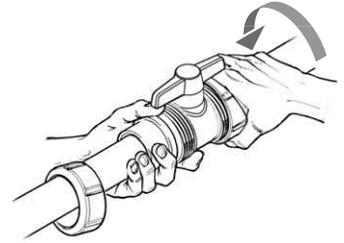
**STEP 8** Attach final Union Nut to Valve Body.
