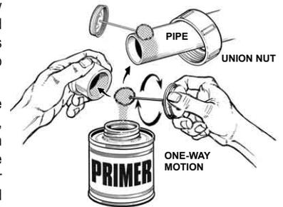
Apply primer to the outside of pipe ends in the same manner extending application area to slightly beyond the insertion depth of the End Connector Socket. Apply a second coat to both pipe and socket.
