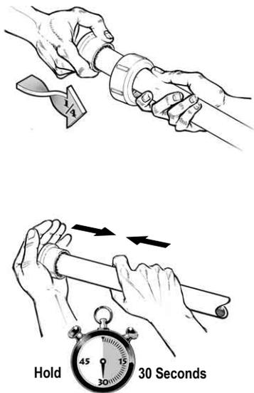
Repeat STEP 6 to attach opposite end connector to pipe and branch on 3-Way Valves.
