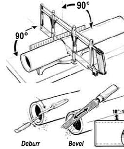
**STEP 1** Pipe Preparation - Prepare connecting pipes as required. Pipe ends must be cut square at 90° using a wheel type cutter or a saw and miter box.
