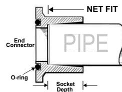
Interference must occur between 1/2 the Socket depth (FULL INTERFERENCE) and the Socket bottom (NET FIT). Do not use components which do not properly mate.
