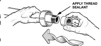
**STEP 3** Wrench Make Up - Threaded pipe and valve components must always be installed using commercially available strap wrenches. Do not use conventional pipe wrenches, which can cause damage to plastic piping materials. Apply wrench make-up of no more than 1 to 2 turns beyond finger-tight thread engagement. Care must be taken in final positioning so as to avoid the need to "Back-up" the wrench assembly.
