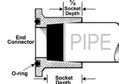
**STEP 3** Check the Joint Interference fit between the pipe and the End Connector Socket. An Interference Fit is necessary for proper fusion of the joint. To check, lightly insert the End Connector Socket over the prepared pipe ends. DO NOT FORCE THE SOCKET ONTO THE PIPE.
