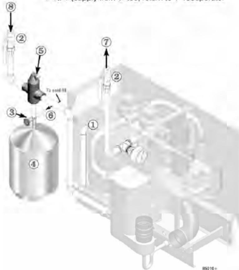
**NOTICE** Pipe diaphragm- or bladder-type expansion tanks to the bottom of the separator.
