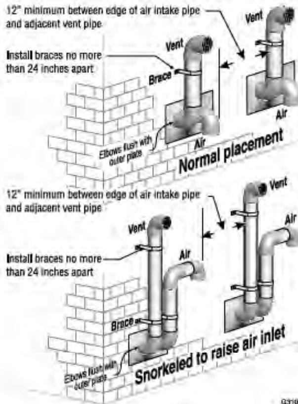
**Figure 49** Sidewall termination assembly — using separate pipes
