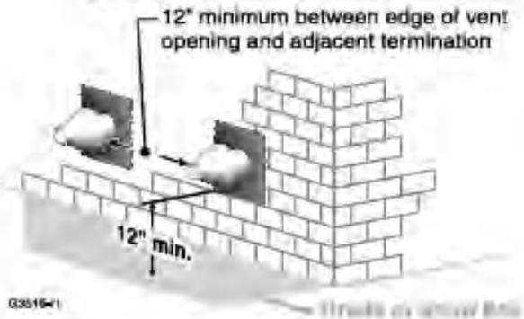
**Figure 52** Installing and supporting the concentric sidewall vent assembly
