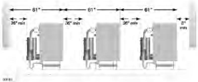
**Figure 29** Back-to-back installation of multiple GV90+ boilers, showing RECOMMENDED clearances
