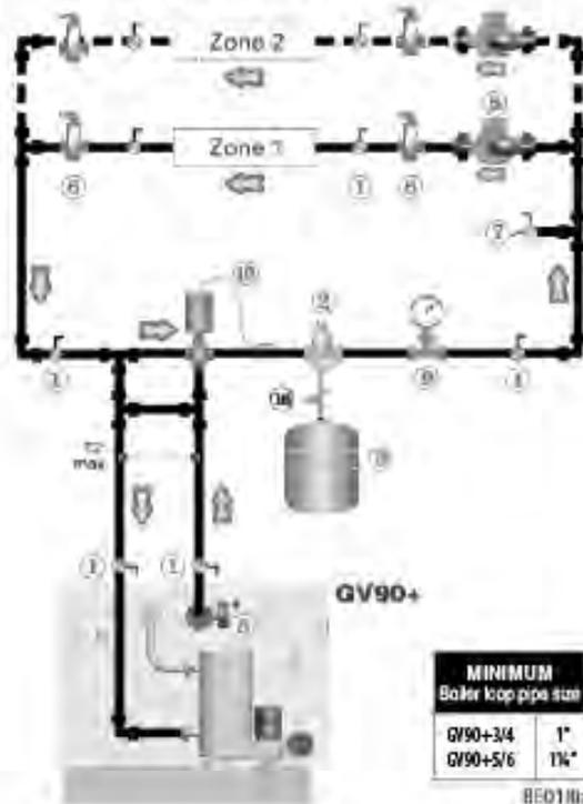
**Figure 24** Auto system supply temp regulation — circulator zoning
