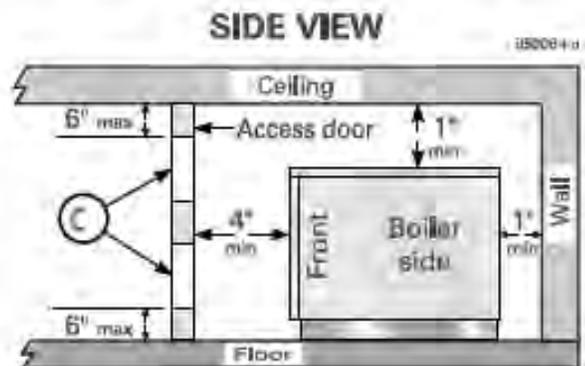
**WARNING NOTICE SPECIAL REQUIREMENTS FOR AIR OPENINGS:** For installations with clearances less than recommended service clearances (Figure 2, page 6), but **no less than shown in Figure 4** — An access door must be provided, fitted with two air openings as shown in Figure 4. Each opening must have a free area no less than 1 square inch per 1000 Btuh input of the GV90+ boiler in the space. **DO NOT apply the air opening sizes given in Figure 42, page 36 or Figure 60, page 50.**
