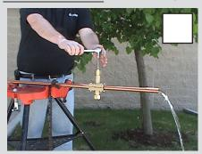
Use a 3/8" socket wrench, manual operation only! Do NOT use a drill motor.
