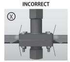
Uneven gap distribution can lead to install failure
