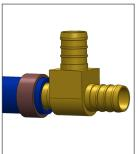
Fitting not inserted completely into tube end.
