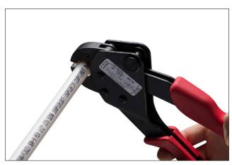
4. Compress tool perpendicular to tube. Compress only once. Remove defective connections. Use a gauge to assure a proper joint. Test all completed joints.
