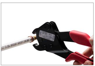
3. Position ring over sealing barbs of the fitting. The ring should be positioned approximately 1/8" to 1/4" from the end of the tube.
