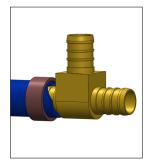
Tube not cut squarely – ring not compressing tube for a secure seal.
