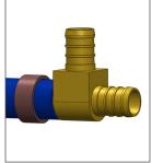
Ring placed too far forward or too far back & not positioned over sealing barbs of fitting.
