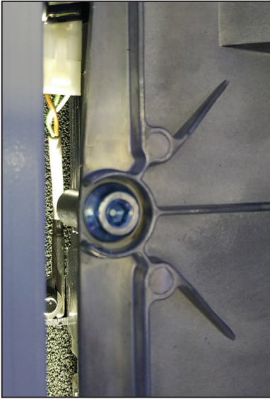
Figure 33: Heat exchanger temperature sensor
