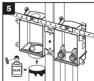
Connect drain pipe. Apply glue to pipe only
