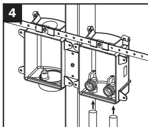
Connect supply lines according to industry standards. Open valves before any soldering
