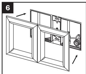
Remove test cap over drain line and install frame after wall finish
