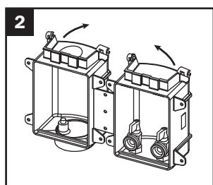
Squeeze and bend clip slightly to hold the stud.
