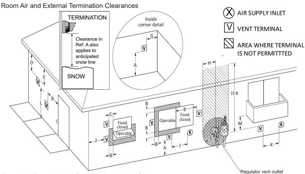
Figure 38: Room Air and External Termination Clearances
