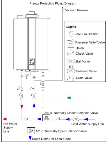
Figure 7: Freeze Protection Piping Diagram
