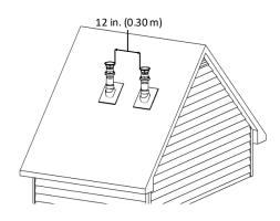
Figure 25: Between terminals at same level
