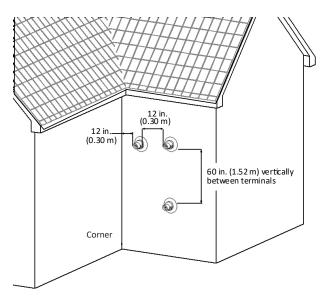
Figure 22: Concentric Pipe Termination Clearances
