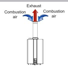
Figure 23: Concentric Pipe
