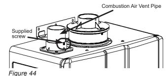
4. Place the vent screen or room air screen inside elbow and secure with the supplied screw. Use the room air screen for environments where room air is dusty (Figure 45). Vent Screen
