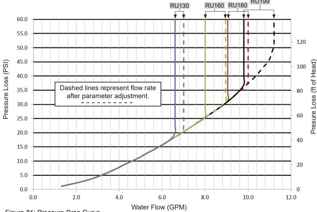
Figure 81: Pressure Drop Curve
