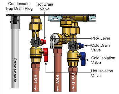
Figure 77: Piping Diagram
