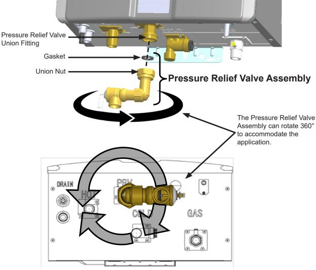
Figure 53: Pressure Relief Valve Assembly
