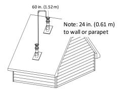
Figure 24: Between terminals at different levels
