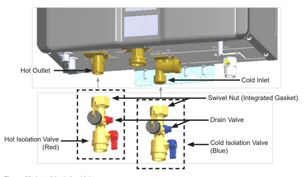
Figure 52: Install Isolation Valves
