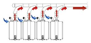
Figure 20: Common Vent, Room Air
