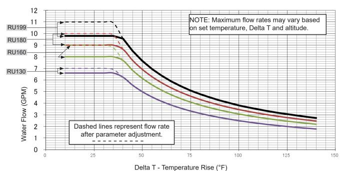
Figure 82: Water Flow Curve
