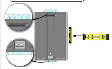
Figure 13: Mount water heater
