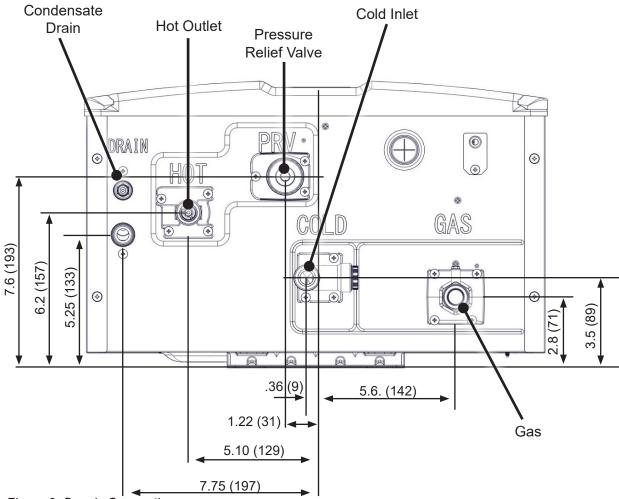
Figure 6: Supply Connections
